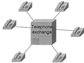
Figure 1.2. The example of the telephonic network with six telephone subscribers and a switching node
