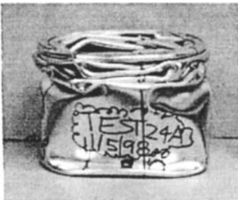
Figure 7 (a) Typical failed empty aluminium alloy tube
