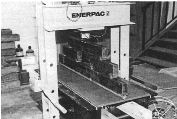
Figure 4: Cemboard specimen being tested for modulus of elasticity
