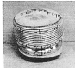
Figure 7 (b) Typical failed aluminium alloy tube with foam filling
