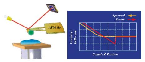
**Fig. 11.26** AFM apparatus configuration (*left*) and representative graph of standard AFM adhesion force curves. *Orange* and *red lines* are for cantilever tip approach and retraction from a substrate, respectively
