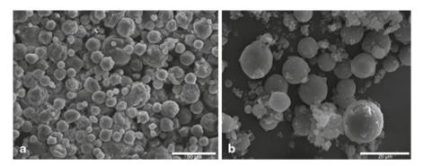
**Fig. 6.9** Example polyanhydrides microspheres made by cryogenic atomization. **a** 50:50 CPH:SA, scale bar represent 50 μm. **b** 80:20 CPTEG:CPH, scale bar represent 20 μm. (Reproduced from Lopac et al. [41] by permission of John Wiley & Sons (copyright 2009))
