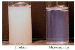
Particle Size :  $\sim 400 \text{ nm}$   $\sim 30 \text{ nm}$ Surface Area :  $\sim 15 \text{ m}^2/\text{ml}$   $\sim 215 \text{ m}^2/\text{ml}$
