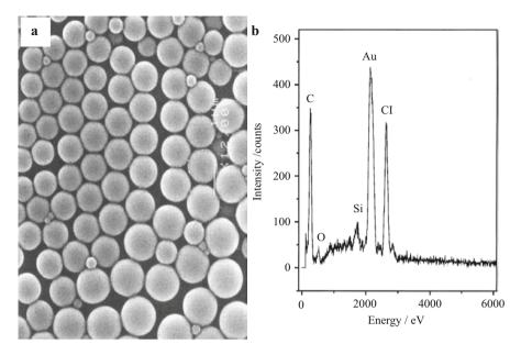
**Fig. 2.19 a** SEM of spherical loratadine particles coated with a silica layer, when 0.08 g of "active" silicic acid was added to 1 g of the dispersion (described in Sect. 2.4.4) and **b** the EDS analysis of the same particles. [51]
