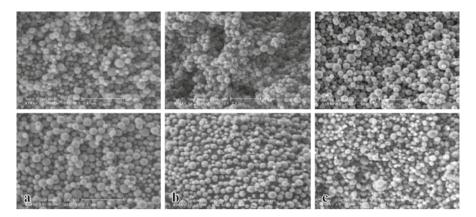
**Fig. 6.5** SEM images of poly(ester-anhydride) microparticles made with the W/O/W double emulsion technique. *Top row*: initial microspheres. *Bottom row*: PBS degraded microspheres (in PBS solution for 3 days). **a** 0% polyanhydrides, **b** 50% polyanhydrides, **c** 100% polyanhydrides. (Reproduced from Pfeifer et al. [43] by permission of Elsevier Ltd (copyright 2005))
