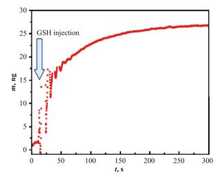
Au/PoPD(GSH) sensor are presented. The total mass of the polymer template film with embedded GSH was  $\Delta m = 274$  ng ( $\Delta f = 238$  Hz).
