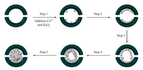
Fig. 7.4 Growth of hollow nanoparticles of Co<sub>3</sub>O<sub>4</sub> in the interior cavity of apoferritin
