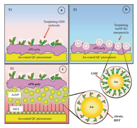
**Fig. 9.15** Schematic of GSH-templated sensor designs: **a** GSH embedded in a PoPD polymer film (oPD-poly) on a Au piezoelectrode (sensor T1), **b** AuNP-SG nanoparticle-templated PoPD film on a Au piezoelectrode (sensor T2), and **c** GSH embedded in a PoPD film electrodeposited on a layer of AuNP network assembled on a SAM of MES on a Au piezoelectrode (sensor T3) (from [35], with permission from the Electrochemical Society)
