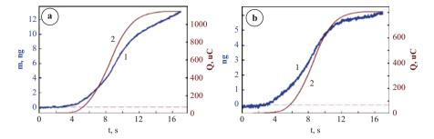
Fig. 9.17 Apparent mass (1) and charge (2) consumed in electropolymerization of a PoPD template from 5 mM oPD+10 mM GSH in 10 mM phosphate buffer by potential scanning between  $E_1 = 0$  and  $E_2 = +0.8$  V at a scan rate of v = 100 mV/s: a 1-st cycle, b 17-th cycle (from [35], with permission from the Electrochemical Society)
