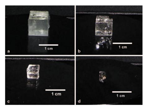
**Fig. 6.2** Crosslinked thiol-ene polyanhydride cube (made with 1:1 functional group stoichiometry of PETMP and PNA, with 0.1 wt.% 1-hydroxycyclohexyl phenyl ketone as the photoinitiator) after **a** 0 h, **b** 18 h, **c** 48 h, **d** 72 h in deionized water. (Reproduced from Shipp et al. [36] by permission of The Royal Society of Chemistry (copyright 2009))
