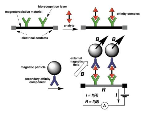
Fig. 5.5 Biosensors based on magnetoresitive materials that provide magneto-electronic transduction of biorecognition events of biomolecules labeled by magnetic nanoparticles
