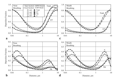
**Fig. 8.5** Comparison of regional deposition results from the ICRP (LUDEP) and the MPPD models for a resting breathing pattern **a** and **b** are for nose breathing; **c** and **d** are for mouth breathing. (Taken from [14])
