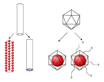
**Fig. 7.9** Synthesis of nanoparticles on viral template. **a** Growth of nanowires on philoviruses; **b** growth of nanocrystals on the end of TMV nanorod; **c** growth of nanoparticles inside a viral capsid; **d** subsequent modification of viral capsid with nanparticle inside
