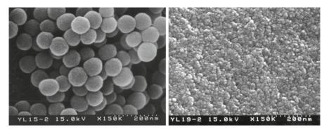
Fig. 11.30 Scanning electron micrographs of two sizes of colloidal silica synthesized by the Stober sol–gel method. Both photos are at 150 K magnification
