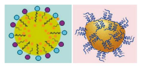
**Fig. 11.2** Representation of a colloidal oil droplet (*yellow*) in water stabilized by surfactants (*blue* and *purple*) and showing absorbed overdosed chemical (*orange*) (*left*); and of a carrier particle with chemical adsorbing functions attached (*blue*) for binding overdosed chemical (*right*)
