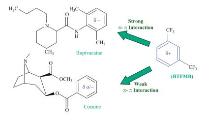
**Fig. 11.23** Selective  $\pi$ – $\pi$  interaction between a smart oil (BTFMB) used for microemulsions and different  $\pi$  donors
