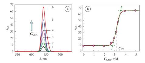
**Fig. 9.2** a Elastic light scattering spectra for 10.1 nM AuNP<sub>5 mm</sub> for different concentrations of GSH, recorded within 1 min of GSH injection, CGSH [mM]: (1) 0, (2) 2.67, (3) 3.0, (4) 3.17, (5) 3.33, (6) 5; **b** Dependence of Isc vs. CGSH; incident beam wavelength:  $\lambda_{ex} = 640$  nm (from [156], with permission from Elsevier)
