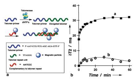
**Fig. 5.11 a** Assembly of the magnetic nanoparticles on the telomeric repeat units generated by telomerase. **b** The change of T2 relaxation time after addition of the oligonucleotide-functionalized magnetic nanoparticles to: (a) the oligonucleotide consisting of 54 telomeric repeat units generated by telomerase; (b) the telomeric-primer without the telomeric repeat units. (Adapted from [127], Fig. 5.1b, with permission.)
