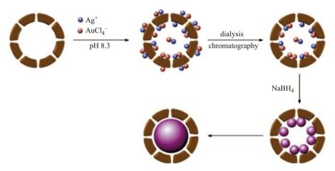
Fig. 7.7 Preparation of Ag-Au alloy nanoparticles through simultaneous treatment with cationic and anionic precursors
