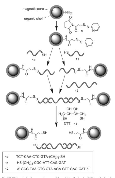
$\textbf{Fig. 5.7} \ \ DNA \ analysis \ using \ magnetic \ nanoparticles \ as \ labels \ allowing \ the \ NMR-transduction \ of \ the \ hybridization \ process$
