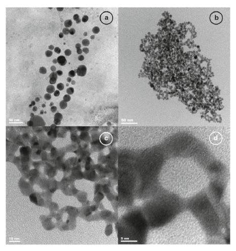
**Fig. 9.8** HR-TEM images of ZONYL-capped gold nsanoparticles before **a** and after assembly with 15  $\mu$ M homocysteine **b**-**d**;  $C_{AuNP} = 6$  nM,  $C_{ZONYL} = 0.22\%$ , pH = 6; bar size: **a** 50 nm, **b** 50 nm, **c** 10 nm, **d** 5 nm (from [152], with permission from Elsevier)
