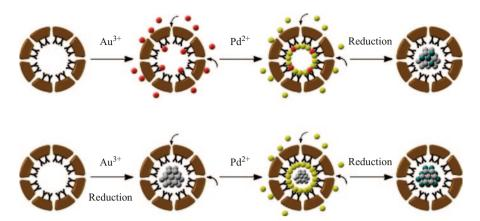
**Fig. 7.6** Preparation of Au/Pd bimetallic nanoparticles in HL apoferritin. Au<sup>3+</sup>, Pd<sup>2+</sup>, Au<sup>0</sup>, and Pd<sup>0</sup> are in *red*, *yellow*, *grey*, and *green*
