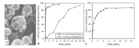
**Fig. 6.8** a SEM image of poly(CPP-SA) (20:80) microspheres loaded with bovine somatotropin (STH), **b** acid orange release from poly(CPP-SA) (20:80) microspheres and polymer degradation, and **c** STH release from poly(CPP-SA) (20:80) microspheres. (Adapted from Mathiowitz et al. [46] by permission of John Wiley & Sons (copyright 1992))
