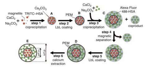
Fig. 10.2 General route for the synthesis of shell-in-shell microcapsules. A initial core, B, coreshell particle, C ball-in-ball particle (type I), D ball-in-ball particle (type II), E shell-in-shell microcapsule. (Reprinted with permission from Ref. [11] Wiley. 10.1002/anie.200701173)
