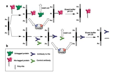
**Fig. 5.4 a** Separation of His-tagged proteins from untagged proteins using magnetic Ni-nanorods. **b** Separation of antibodies specific to polyhistidine (anti-poly-His) from other antibodies using magnetic Ni-nanorods. (Adapted from [71], Scheme 1, with permission).
