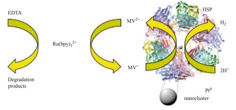
Fig. 7.8 Schematic representation of light mediated production of dihydrogen with platinum nanoclusters inside HSP. Methyl viologen ( $MV^{2+}$ ) is used as an electron transfer mediator between the  $Ru(bpy)_3^{2+}$  photocatalyst and Pt-HSP
