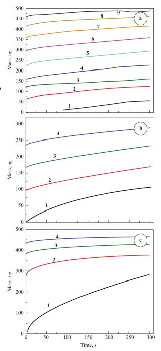
Fig. 9.19 a Chronoamperometric (1) and chronogravimetric (2) transients for the initial electropolymerization stage of a GSH-templated poly(oPD) film T1 on a QC/ Au electrode from 5 mM oPD+10 mM GSH+10 mM HClO<sub>4</sub> solution by a potential step from  $E_1 = 0$ to  $E_2 = +0.8 \text{ V } vs \text{ Ag/AgCl}.$ **b** Apparent mass vs. time response of a T1-type sensor after injection of a free GSH solution (5 mM) (from [35], with permission from the Electrochemical Society)
