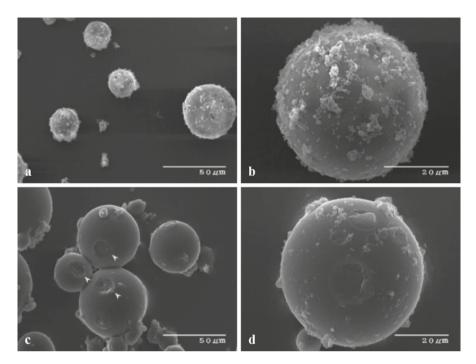
**Fig. 6.6** TT-loaded poly(CPH-SA) microspheres. 20:80 copolymer microspheres showing small polymer particles flocculated on their surfaces [a and b] and 50:50 microspheres with small circular divots [indicated by the *arrowheads* in c] formed when the loosely adhered clumps of microspheres break apart [c and d]. (Reproduced from Kipper et al. [44] by permission of John Wiley & Sons (copyright 2006))
