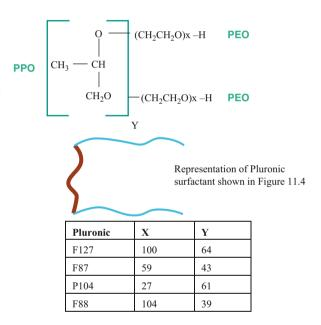
These amphiphilic molecules aggregate and form micelles when mixed with water. However, with oil droplets present Pluronic molecules assemble at the interface between the oil core and water, with the hydrophilic PEO termini extending into the water phase.
