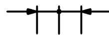
(f) Point (used only if no place for arrowhead; the oblique stroke may also be used – BS 8888)
