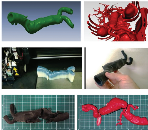
Figure 4. A–D. Sequence of the development of a 3D flexible model of aorta from CT scanner files; E: 3D printed flexible model of aorta positioned on measuring scale table (scale reference: 1 cm 2 ), damaged after tests (3D Printed in “Tango black” flexible resin on OBJET Connex 350)—Instituto Nacional de Tecnologia—Laboratório de Modelos Tridimensionais—Ministério da Ciência, Tecnologia e Inovação.; F: variant colored rigid 3D printed model of aorta (3D printed in thermoplastic ABS—Stratasys U-Print-Fused Deposition Modeling)—Núcleo de Experimentação Tridimensional—NEXT PUC-Rio.
