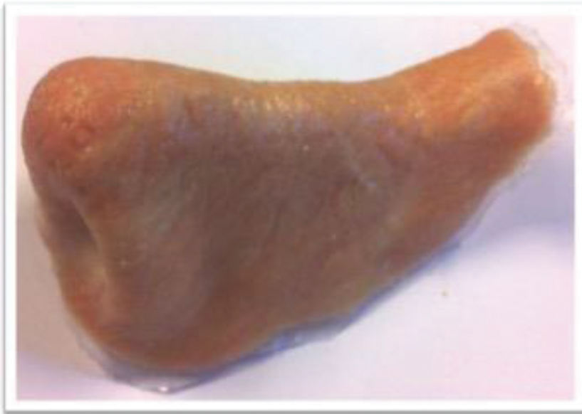
Figure 10. Photograph of a 3D printed nasal prosthesis infiltrated with a compatible medical grade silicone infiltrate (Approx. part Dim: 40 × 24 × 25 mm).
