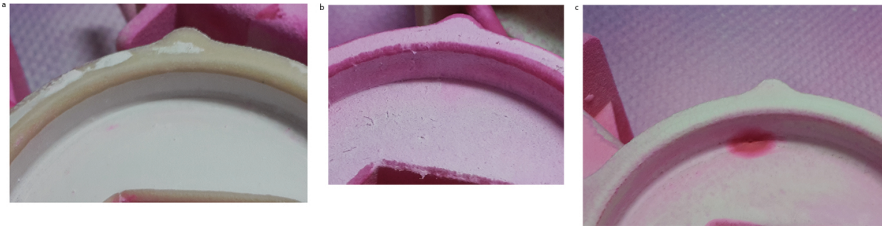
Figure 25. Results of the color penetration test: (a) short immersion, (b) long immersion, and (c) problem areas.
