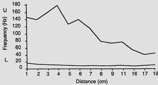
FIGURE 8.5. Distant-dependent changes in the propagation of surface waves. A: Changes in the time waveform of the wave packet at different distances during concentric spreading of the surface wave. B: Lower (L) and upper (U) frequency limits of the surface wave amplitude spectrum as a function of distance. High frequencies attenuate more rapidly with distance, producing a compression of the bandwidth. (From Montgomery et al. 1995b, © Chapman & Hall.)
