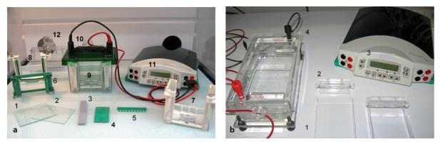
**Fig. 8.6 a, b** (a) *1* Spacer plates; 2 short plates; 3 casting stand gasket; 4 gel releaser; 5 comb; 6 casting frame; 7, 8 clamping frame; 9 buffer tank; *10* lid; *11* power supply; *12* casting stand. (b) *1* UV-transparent tray; 2 comb; 3 power supply; 4 electrophoresis cell
