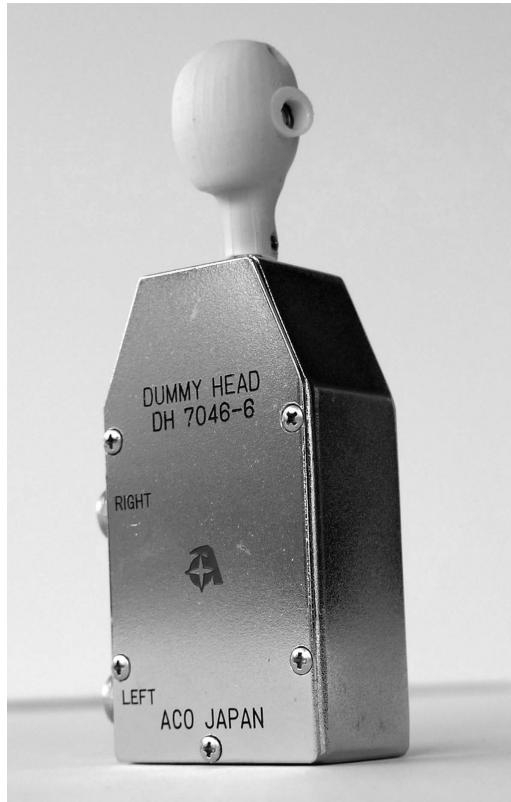
Figure 13.7 An N=10 scale model manikin with microphones behind its pinnae. (Photo by Mendel Kleiner.)
