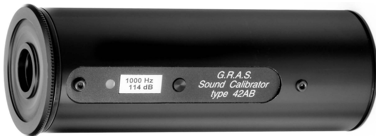
Figure 14.2 A small low internal impedance calibrator for use with standard size cylindrical pressure microphones. Microphone is inserted in the hole at cylinder end on the left. (Photo courtesy of G.R.A.S., Copenhagen, Denmark.)
