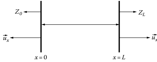
Figure 2.8 Sound propagation between two walls.
