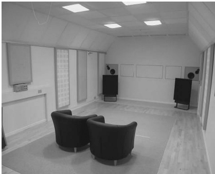
Figure 11.2 The IEC listening room at the Aalborg University Centre's Acoustics Laboratory is a good example of a listening room possibly similar to what may be achieved in a domestic environment. Note the use of diagonal absorbers along upper side walls to reduce low frequency reverberation time. (Photo courtesy of Aalborg University Center [AUC], Aalborg, Denmark.)
