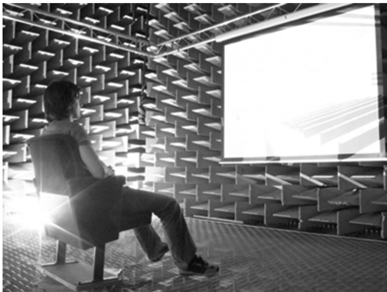
Figure 14.29 Listening tests in an anechoic chamber, combining aural and visual cues. (In a listening test the lights will be switched off and only the screen visible.) (Photo by Pontus Larsson.)
