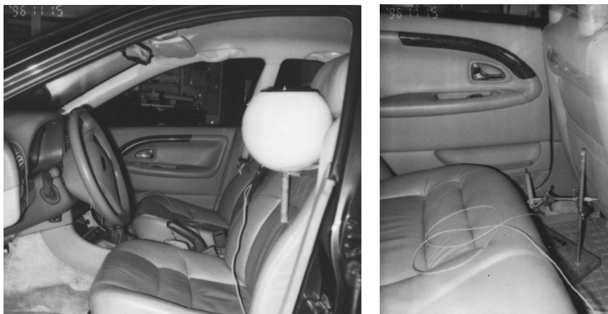
Figure 14.17 In reciprocity measurement, the loudspeaker and microphone locations are interchanged to allow easier testing of suitable loudspeaker positions. The loudspeaker takes the position of the listener's head. (Photos by Mendel Kleiner.)
