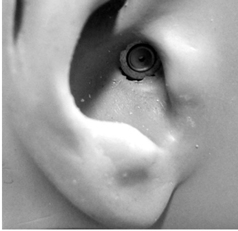
Figure 6.4 A small microphone inserted at the ear canal opening of an ear replica to sense the sound pressure in the concha. (Photo by Mendel Kleiner.)
