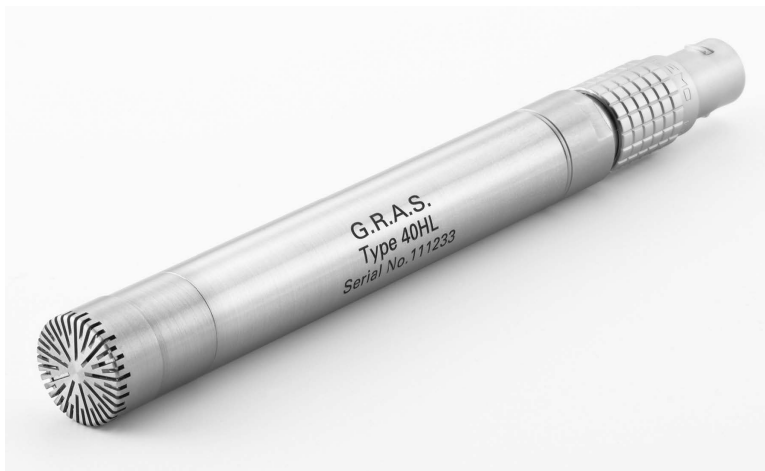
Figure 14.1 Typical 12 mm ( \frac{1}{2} " ) diameter microphone used for sound pressure measurement. (Photo courtesy of G.R.A.S., Copenhagen, Denmark.)
