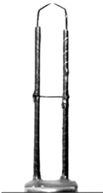
Figure 13.2 A spark gap (at the top of the figure) functions well as an omnidirectional sound source in ultrasonic scale modeling. Gap is about 1 mm wide. (Photo by Mendel Kleiner.)
