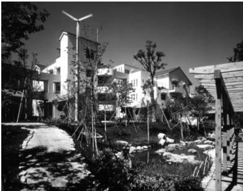
Fig. 19.18 'Biotope Garden' shortly after the completion (April 1997). The Biotope Garden is protected topographically and accommodates a variety of plants, birds and insects. The water from the preserved well is circulated by the wind charger behind, only when enough wind blows
