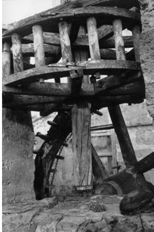
Fig. 15.1 Technology transmission from the East: the Arab noria , a mule-powered water-lifting apparatus with buckets on an endless chain, was introduced to Spain by the Arabs probably in the fourteenth century. This one was still in use six centuries later (Photo: © Paul Oliver)
