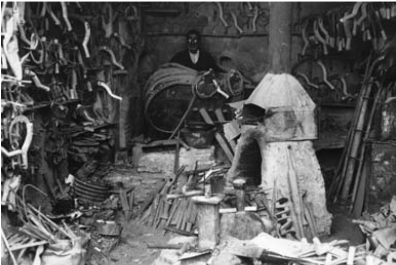
Fig. 15.2 Timeless tools: both his forge and the tools that this Iranian blacksmith has wrought from scrap iron are virtually identical to those made and used in Roman times (Photo: © Paul Oliver)
