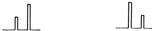
Fig. 41. The signal sequence used by Ronken to measure minimum time resolution for clicks. On each listening trial two such click-like signals were presented. The listener responded only Same or Different. On half the trials the same signal is presented twice. On the other half (randomly determined) the second signal is the reverse of the first. The spacing between the strong and the weak peak is varied from trial to trial. When the time between peaks is so small that the listener can tell the difference only 75 % of the time, we have reached a limit of time resolution for peak spacing. If the amplitude ratio between peaks is changed, the results will differ somewhat
