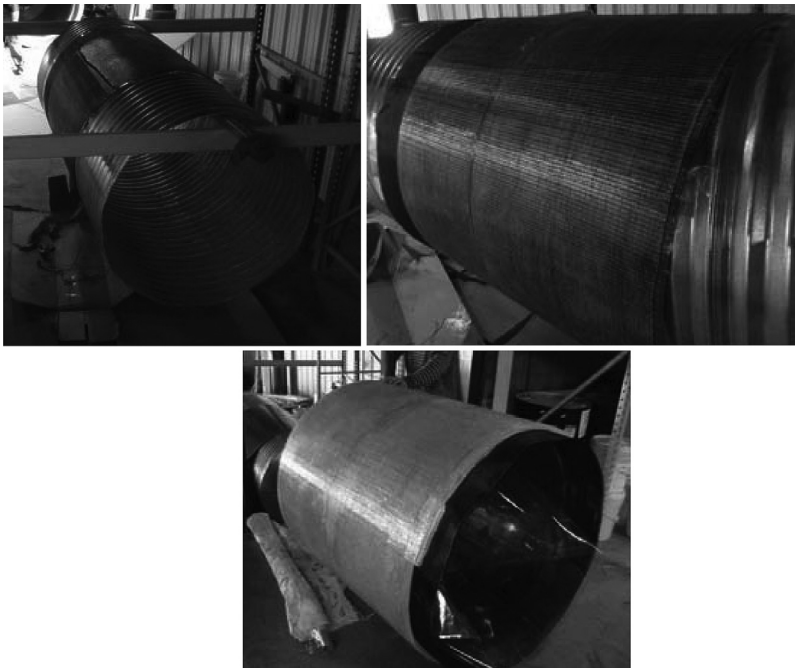
Figure 3.12 Steps in the construction of StifPipe ® : (a) corrugated metal pipe used as mandrel, (b) carbon fabric wrapped around mandrel, and (c) pipe allowed to cure in ambient condition.
