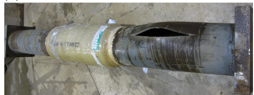
Figure 12.11 (a) Failure of an unrepaired Type A pipe and (b) failure of a repaired Type A pipe showing rupture outside of the repaired region.
