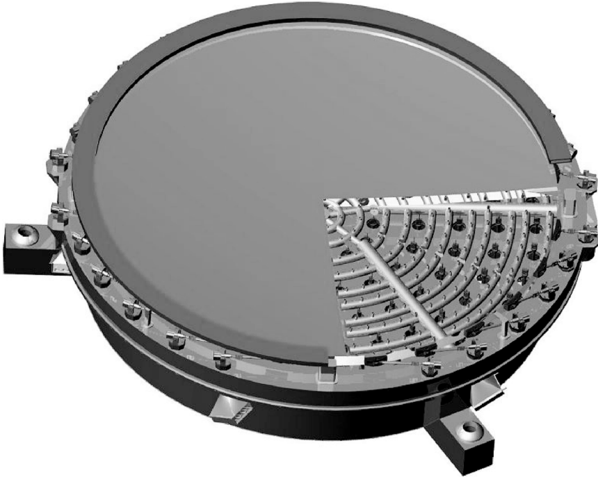
Figure 38.1 The ATST M1 assembly. The thin-meniscus mirror is cut away to reveal the support array and air-cooling distribution network. (Courtesy National Solar Observatory.)
