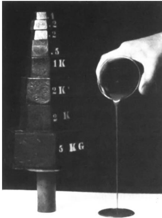
Figure 5.47 Effect of remoulding on the undrained shear strength of a sensitive soil (Leda Clay). (From Crawford, C.B., Géotechnique , 13, 2, 132–46, 1963. With permission.)
