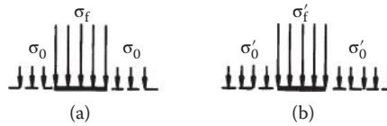
Figure 8.19 Schematic diagram of vertical stresses below and to one side of foundation base: (a) short-term analysis; (b) long-term analysis, Example 8.3.
