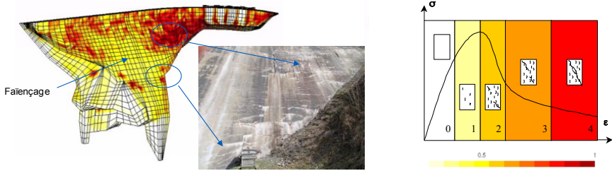
Figure 8. Comparison between evaluated damage and observed cracking pattern
