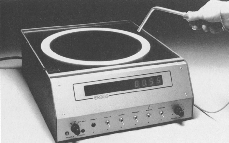
Figure 1.3 Pursuit rotor task (Forth Instruments, Livingston, Scotland) used to assess perceptual-motor learning. The subject has to follow the moving light by holding the stylus tip over the light source. A tone is emitted while the stylus is over the target. The speed of the target can be controlled, and time-on-target for each trial is indicated on the display panel. Such a task is often performed well by neurological patients who otherwise have marked impairment on more traditional memory tests
