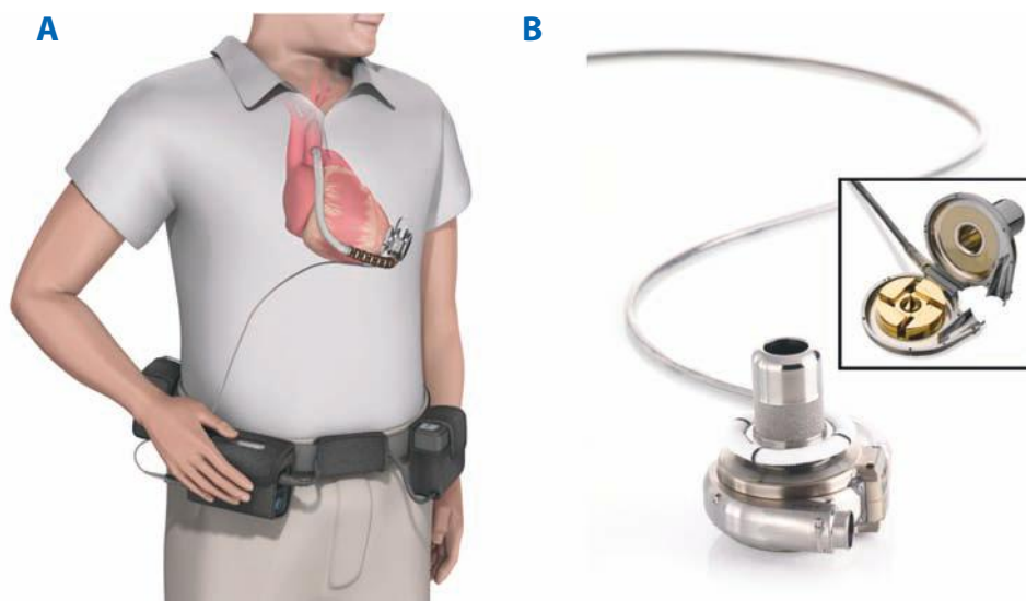
Figure 21-13. The HeartWare HVAD system. A. Both the device controller and batteries are held in a wearable carrying case and connected to the ventricular assist device through the driveline. B. The main component is a centrifugal blood pump, called the HVAD, which is implanted within the pericardium. The only moving part in the device, the impeller, is suspended within the pump using magnets and thrust bearings. Similar to the HeartMate II, it can deliver a flow rate of up to 10 L/min. (Images reproduced with permission from HeartWare.)
