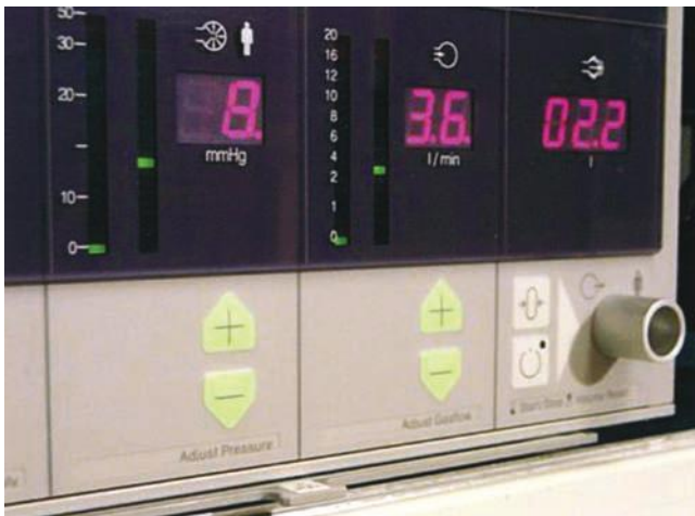
Figure 14-6. It is essential to be able to interpret the insufflator pressure readings and flow rates. These readings indicate proper intraperitoneal placement of the Veress needle.
