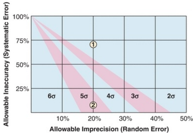
FIGURE 4.7 OPSpecs chart used to determine process performance. The allowable imprecision is plotted against the allowable inaccuracy as percentage of the total allowable error. Assay performance changing from point 1 to point 2 by reducing inaccuracy improves the performance from a 2σ process to a 5σ process.
