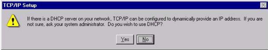
Fig 11.7 Confirmation for dynamically configuring TCP/IP
