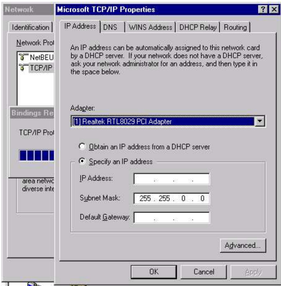
Fig 11.8 Specifying static IP Address
