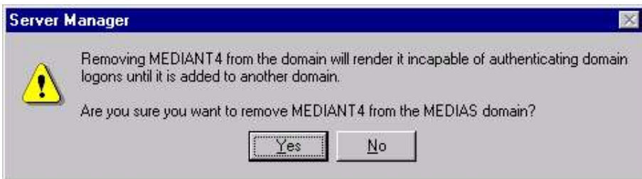
Fig 14.3 Removing domain from Server Manager
