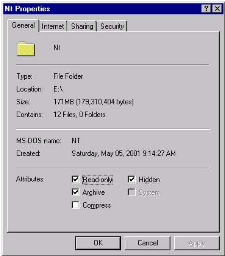
Fig 10.2 Setting Folder properties on NTFS
