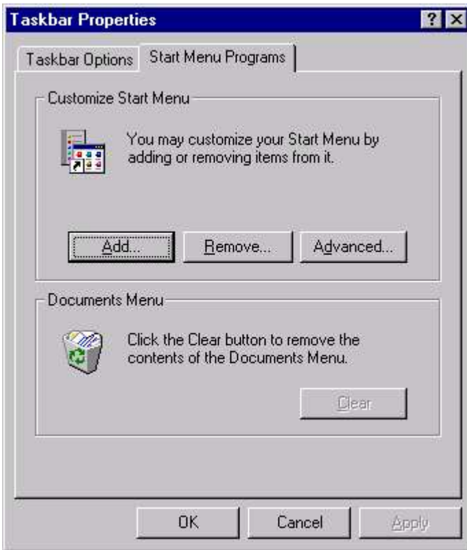
Fig. 4.14 Start Menu tab of Taskbar Properties
