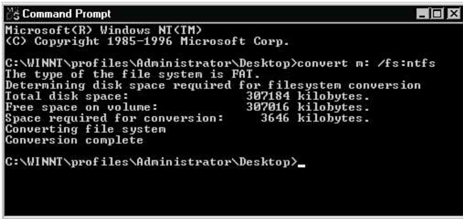
Fig 6.1 Converting to NTFS using Convert command
