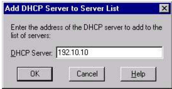
Fig 12.4 Adding DHCP server to Server List
