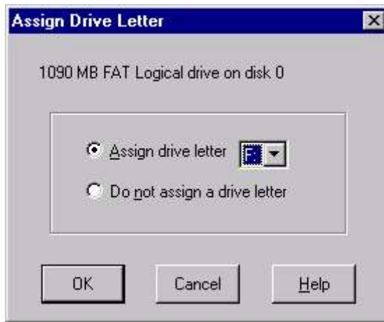
Fig 6.12 Assigning Drive Letter to the partition
