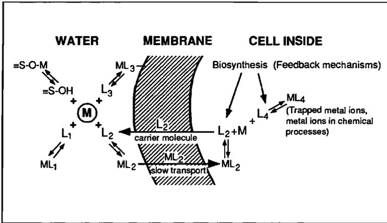
Figure 8. Uptake model in a simplified model, the metal ions equilibrate on the outside of the cell with biologically produced and excreted ligands  $L_2$  or ligands on the cell surface  $L_3$ ; these reactions are followed by a slow transport step to the inside of the cell. In the cell, the metal ions may be used in biochemical processes or become trapped in inactive forms as a detoxification mechanism. (From Sigg, 1987)
