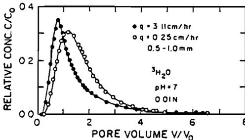
Figure 6. Observed <sup>36</sup>Cl effluent curves showing the effect of pore water velocity on the displacement process.
