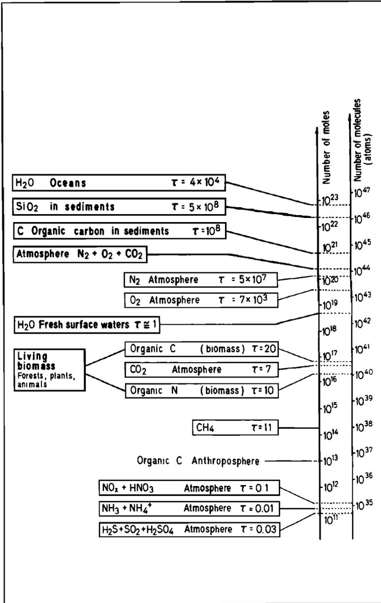
Figure 2. Comparison of global reservoirs. The reservoirs of atmosphere, surface fresh waters and living biomass are significantly smaller than the reservoirs of sediment and marine waters. The total groundwater reservoir may be twice that of fresh surface water. However, groundwater is much less accessible ( $\tau$  = respective residence time [years] of molecule [atoms]) (Stumm, 1986).
