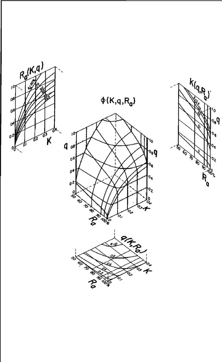
Figure 3. General reservoir storage-yield function  $\phi(K, q, R_a)$ .  $K$  - over-year storage (as fraction of mean annual runoff volume);  $q$  - draft (as fraction of mean flow);  $R_a$  - reliability (annual) = probability of non-failure year<sup>24</sup>.
