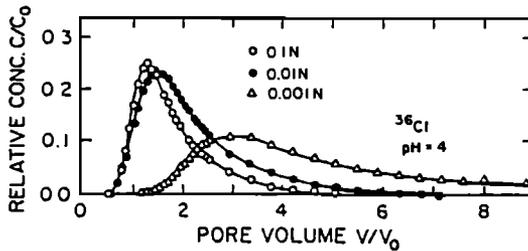
Figure 4. Observed  $^{36}\text{Cl}$  effluent curves showing the effect of total ionic concentration on the displacement process.
