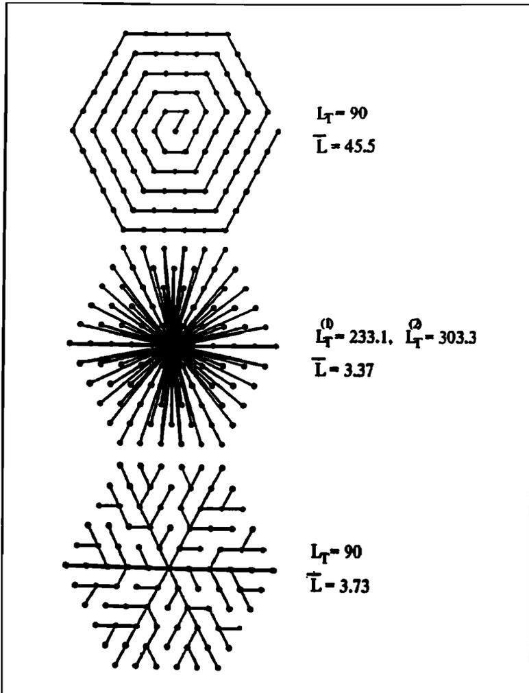
Figure 1. Different patterns of connectivity of a set of equally spaced points to a common outlet.  $L_T$  is the total length of the paths, and  $\bar{L}$  is the average length of the path from a point to the outlet. In the explosion case  $L_T(2)$  refers to the case when there is a minimum displacement among the points so that there is a different path between each point and the outlet [from Stevens, 1947].
