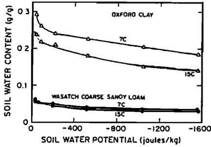
Figure 10. Soil water retention curves for two soils at two temperatures [after Taylor, 1958].
