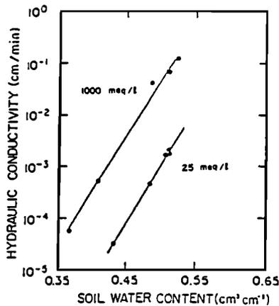
Figure 8. The impact of water quality on the value of the unsaturated hydraulic conductivity.
