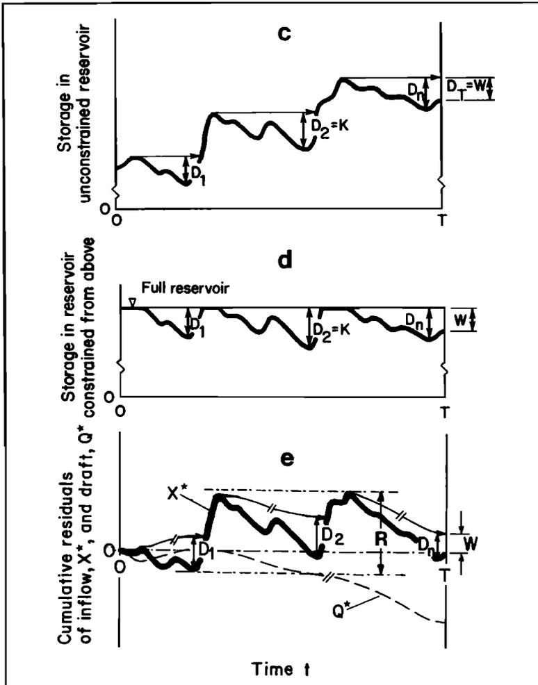
Figure 2—continued. Definition sketch for various types of mass curves used for the determination of storage capacities ( $D_1$ ,  $D_2$ ,  $D_3$ ) required in different periods to meet prescribed reservoir draft.
