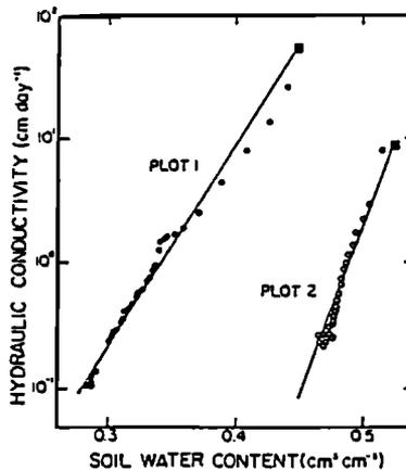
Figure 2. Hydraulic conductivity as a function of soil water content measured at the same soil depth in two plots separated by 50 m.
