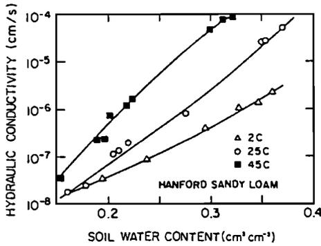
Figure 11. Unsaturated hydraulic conductivity  $K$  as a function of water content  $\theta$  at three temperatures [after Constantz, 1982].
