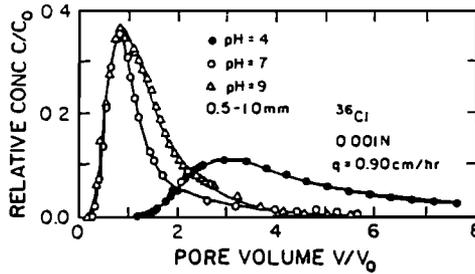
Figure 5. Observed <sup>36</sup>Cl effluent curves showing the effect of solution pH on the displacement process.
