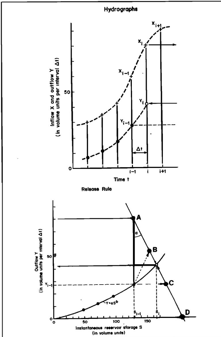
Figure 1. Common principle of reservoir routing methods: To find a position of the water-balance straight-line (whose angle  $\alpha$  is given by the chosen volume scales) such that the difference between inflow and outflow in interval  $\Delta t$  is equal to the change in storage and the outflow obeys the release rule function. One point is needed to fix this position. Examples of points employed: A - Kleměš, B - Sorensen, C - Urban, D - Puls<sup>5</sup>.
