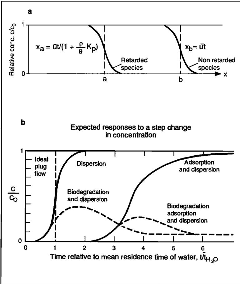
Figure 7a. Advances of adsorbed and non-adsorbed solutes through a column of porous materials. Partitioning of species between solid material and water is described by  $K_p$ . The relative velocity is given by:
