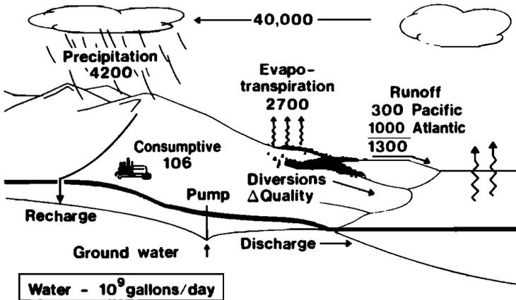
Figure 1. Schematic diagram of the Hydrologic Cycle for the conterminous United States.
