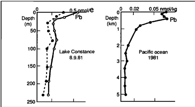
*Figure 10.* Lead profiles in Lake Constance (Summer 1981 data: Sigg, 1985) and in the Pacific Ocean (1981 data: Schaule and Patterson, 1981). The similar shape of these profiles, despite the difference in length scales (kilometers for the ocean and meters for the lake), illustrates the influence of the atmospheric deposition on the upper layers and the scavenging of Pb(II) by the settling particles (Modified from Sigg, 1985).
