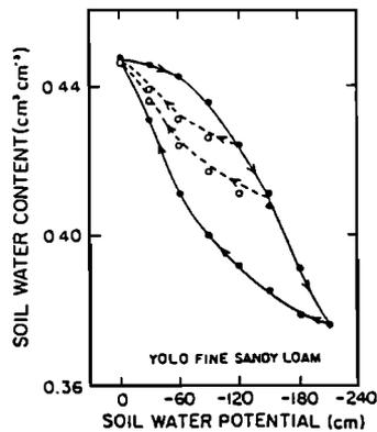
Figure 9. Soil water retention curves. Arrows indicate the direction at which the values of  $\psi$  are decreasing or increasing.
