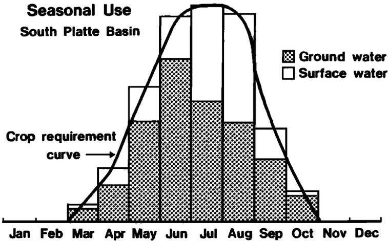
Figure 2. Crop requirement and sources of supply for the South Platte Valley in Colorado. The surface water available does not meet crop demand.
