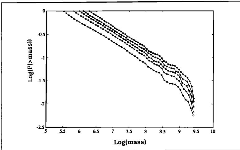
Figure 8. Cumulative distribution of discharges for the same basin as a function of the support threshold.
