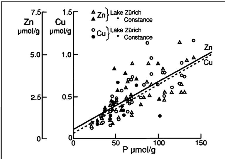
Figure 9. Concentrations of Cu and Zn as a function of P (phosphorus) in the settling material from Lake Zurich and Lake Constance. P serves as an indicator for the quantity of biological material present. The regression lines for Zn and Cu fall nearly together, indicating that rather constant ratios Cu : Zn : P are found in this material (From Sigg et al., 1987).
