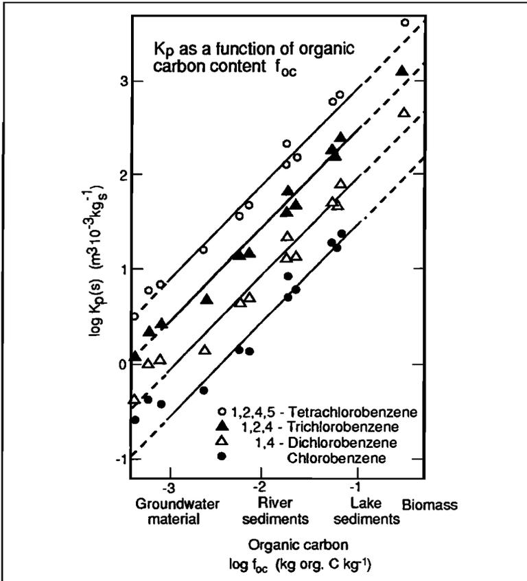
Figure 6 . The distribution of organic substances between water and representative solid materials of different organic carbon content,  $f^{oc}$  (Modified from Schwarzenbach and Westall, 1981).
