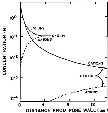
Figure 3. Distribution of monovalent cations and anions near the surface of a clay particle.
