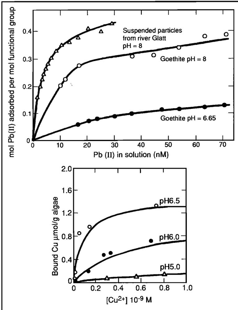
*Figure 4a.* Adsorption of heavy metal ions to the surface of goethite and natural particles. Surface complex formation of  $\text{Pb}^{2+}$  on goethite and the surface of natural particles (Glatt River). The data are interpreted in terms of Langmuir adsorption isotherms.
