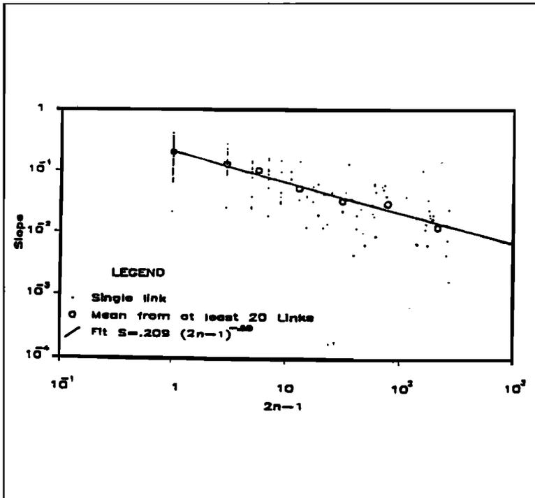
Figure 4. Link slopes as function of magnitude for Big Creek, Idaho [from Tarboton et al. (1991)].
