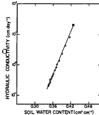
Figure 1. Measured values of soil hydraulic conductivity versus soil water content.
