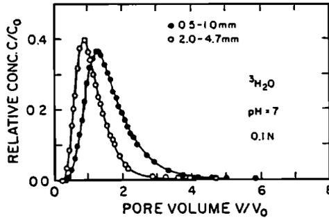
Figure 7. Observed  $^3\text{H}_2\text{O}$  effluent curves showing the effect of aggregate size on the displacement process.
