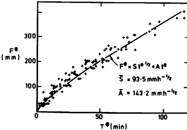
Figure 5. Soil similarity applied to infiltration data.
