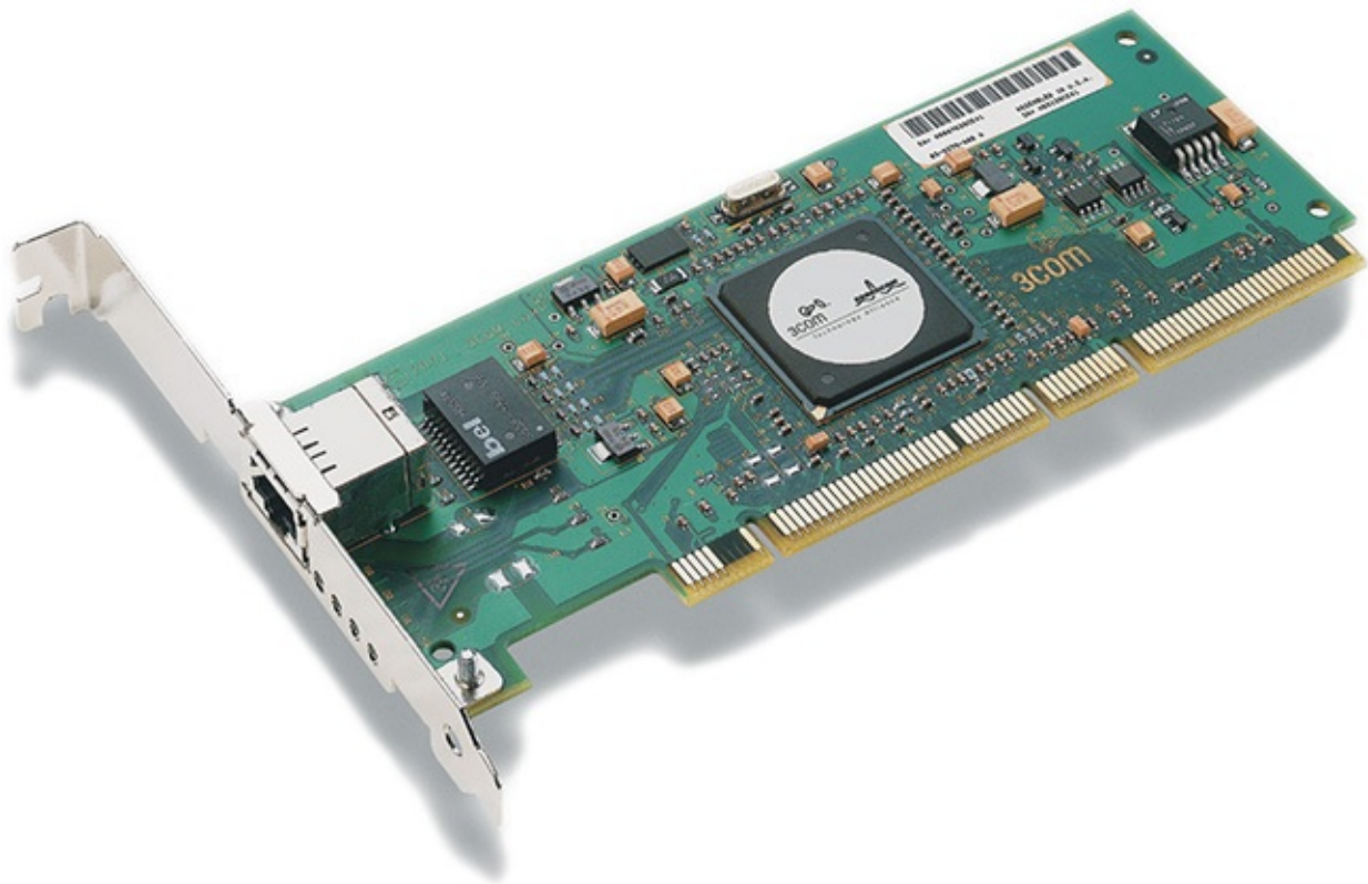
FIGURE 1-8 A 3COM network interface card (courtesy of 3Com Corporation).
