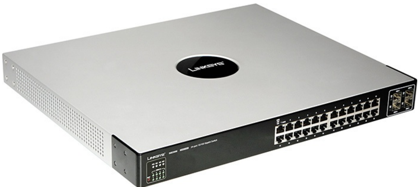
FIGURE 1-13 Linksys 24-Port 10/100/1000 Gigabit Switch (courtesy of Linksys).
