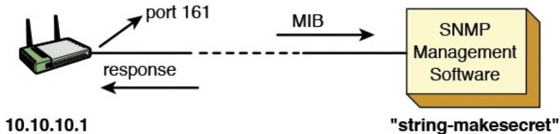
FIGURE 8-4 The setup for connecting the SNMP management software tool to the router.
