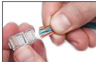
FIGURE 2-25 The clipped wires ready for insertion into the RJ-45 (8P8C) plug.
