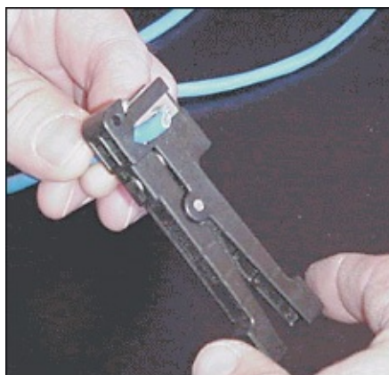
FIGURE 2-23 An example of using the cable jacket stripper to remove the insulation.
