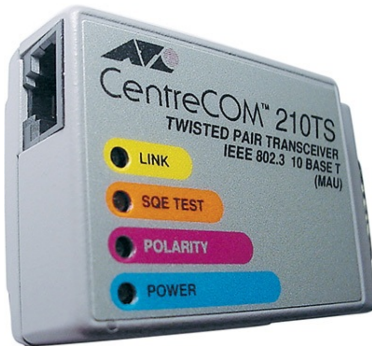
FIGURE 5-17 A CentreCom 210TS AUI to RJ-45 media converter.
