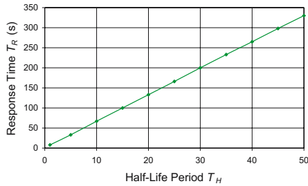
Fig. 3. Correlation of EBAC memory with half-life period T_H and EBAC response time T_R for decreasing traffic intensity
