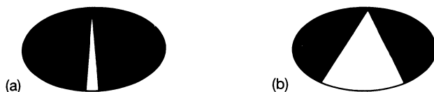
Fig. 4.4 Opening the vocal cords. (a) When lightly closed, the cords vibrate. (b) When spaced apart, the airflow is unimpeded.
