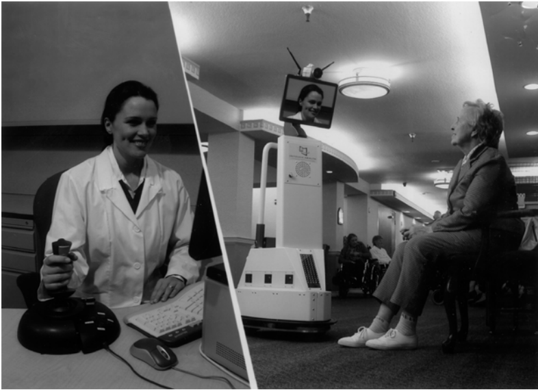
Figure 14.5. “Companion” telehealth robot. The remote clinician (left) is able to control the robot using a joystick. (Source: InTouch Health.)
