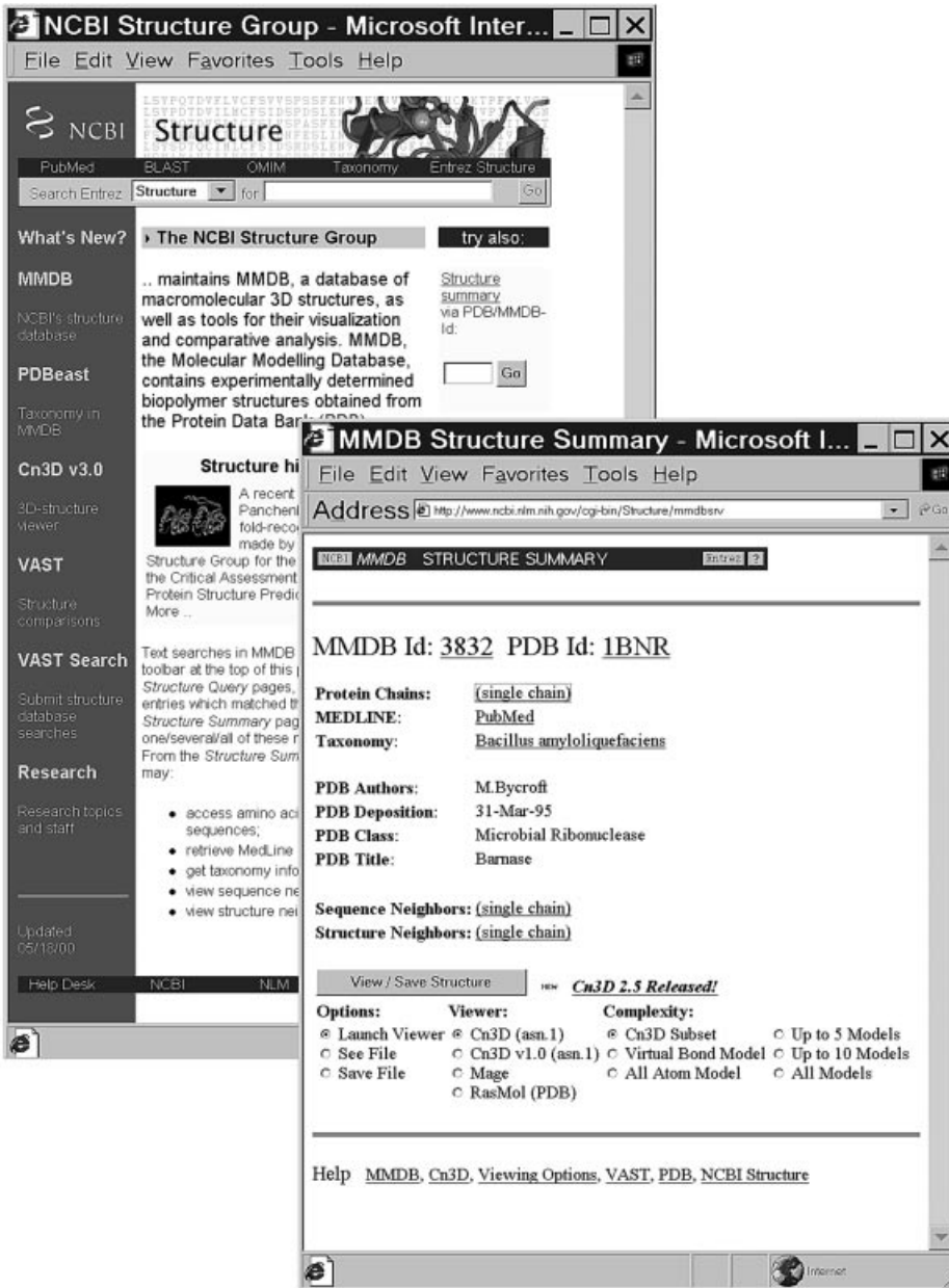
Figure 5.4. Structure query from NCBI with the structure 1BNR (Bycroft et al., 1991). The Structure Summary links the user to RCSB through the PDB ID link, as well as to validated sequence files for each biopolymer, sequence, and three-dimensional structure neighbors through the VAST system. This system is more efficient than the RCSB system (Fig. 5.2) for retrieval because visualization, sequence, and structure neighbor links are made directly on the structure summary page and do not require fetching more Web pages.
