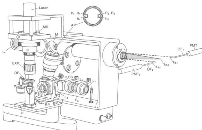
**Figure 19–5.** Fundus camera based bidirectional LDV system. See text for details. (From Riva, C.E., B.L. Petrig, R.D. Shonat, and C.J. Pournaras. *Appl Optics* 28:1078–1083, 1989.)
