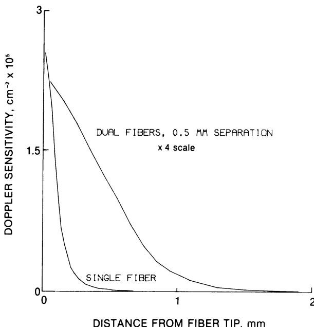
**Figure 7-5.** One-dimensional plot of calculated Doppler sensitivity fields of single-fiber and two-fiber Doppler systems, as a function of distance from the plane containing the tips of the fiber(s). Sensitivity extends farther from the fiber tips for the two-fiber system.
