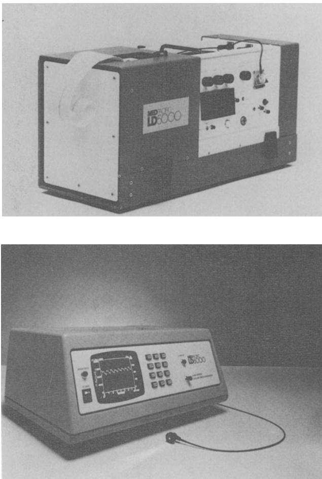
**Figure 3–1.** Medpacific LD-5000 (upper) and LD-6000 (lower) laser-Doppler flowmeter systems.
