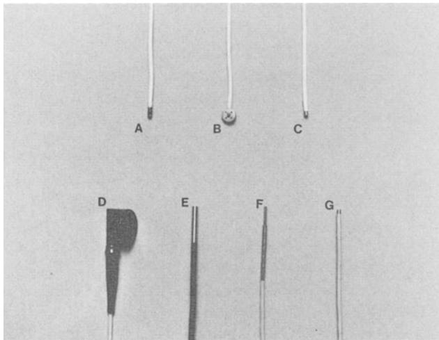
**Figure 5–6.** Fiber optic blood flow probes. A. Implantable prism probe. B. Implantable disk probe. C. Endoscope probe. D. Right-angle probe. E. Hardtip pencil probe. F. Needle probe. G. Softtip pencil probe.
