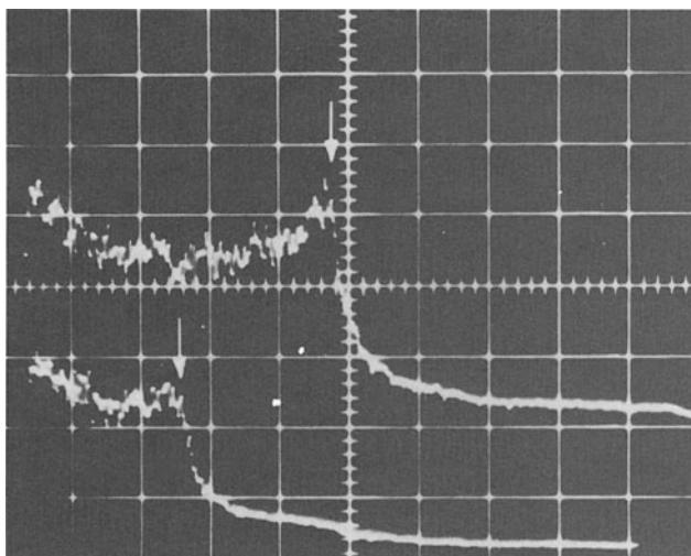
**Figure 19–6.** Doppler shift power spectra (DSPS) from  $0.3\text{ }\mu\text{m}$  polystyrene spheres suspended in water flowing through a  $200\text{ }\mu\text{m}$  internal diameter glass capillary tube. The tube was mounted in the focal plane of a Topcon model eye. Arrows indicate the cutoff frequencies,  $\Delta f_1$  and  $\Delta f_2$ .
