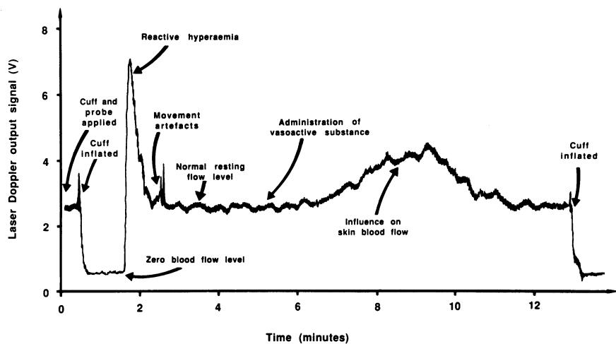
**Figure 4-6.** Recording of blood flow by laser-Doppler flowmetry in a stimuli-response experiment.
