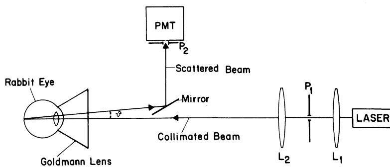
**Figure 19–2B.** Optical system used for recording the power spectrum shown in figure 19–2A. The Goldmann lens is a contact lens to eliminate refraction of light at the cornea. To obtain the spectrum, the signal from the photodetector (PMT) was amplified and then analyzed by a spectrum analyzer. (From Riva, C.E., B. Ross, and G. Benedek. 1972. Invest Ophthalmol Vis Sci 11:936–944.)
