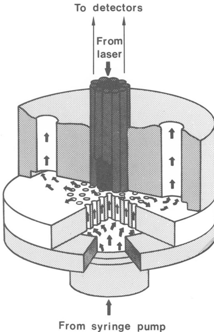
**Figure 4-5.** Flow simulator for evaluation of the performance of laser-Doppler flowmeters (reproduced from [5] with permission of the Institute of Electrical and Electronics Engineers, Inc.).
