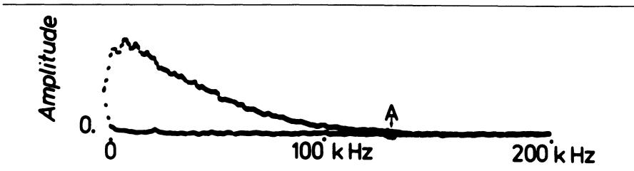
**Figure 7-1.** Homodyne Doppler spectrum obtained from a single fiber, enclosed in a 1 mm catheter and inserted into a flowing stream of whole blood. The upper spectrum is from flowing blood, and the lower spectrum shows system noise at zero flow. Point A is the *maximum Doppler frequency*, defined as the frequency above which the flow spectrum is indistinguishable from noise. (From Kilpatrick et al. [3], figure 3.)
