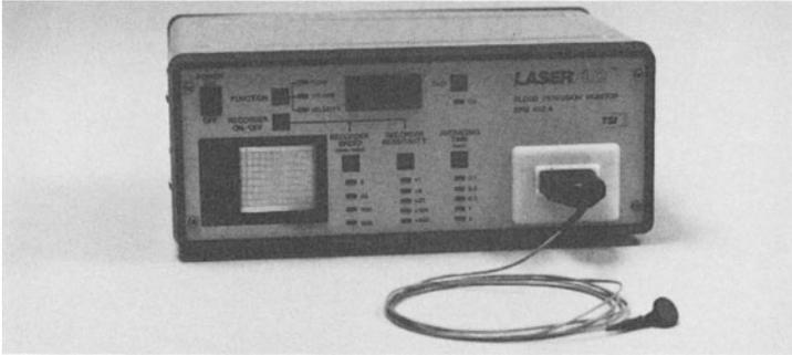
**Figure 5-1.** The Laserflo Blood Perfusion Monitor.
