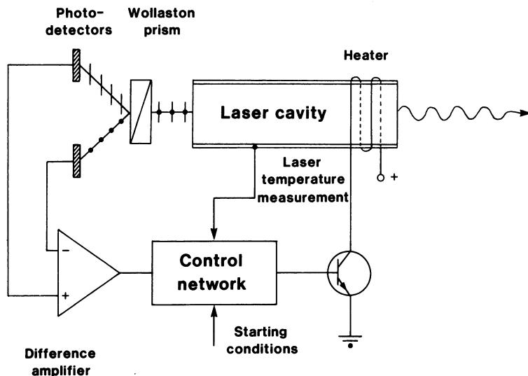
**Figure 6-11.** Block diagram of the principle for laser temperature stabilization. This type of stabilization can substantially increase the signal-to-noise ratio. (From [14] with permission from the International Federation for Medical and Biological Engineering.)
