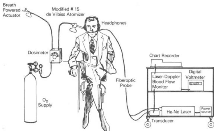
**Figure 14–1.** General configuration of the NIH prototype laser-Doppler flowmeter as adapted for nasal use, shown together with system for topical nasal provocation challenge using nebulized solutions.
