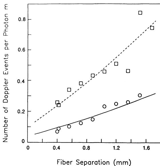
**Figure 2–9.** Average number of photon collisions with moving red blood cells versus distance along the surface of human forearm skin, measured with a laser blood-flow monitor. Data were obtained with a probe with variable spacing between fibers ( $\circ$ , resting skin;  $\square$ , vasodilated skin). (Reproduced from [18].)
