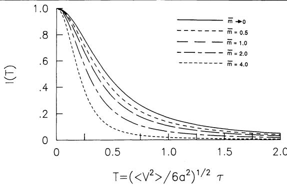
**Figure 2-4.** Normalized photon autocorrelation function, based on equations 2.12 and 2.15, showing the effect of multiple collisions with moving RBCs (different values of  $\bar{m}$ ). Curves are plotted as a function of the reduced variable given in equation 2.14.
