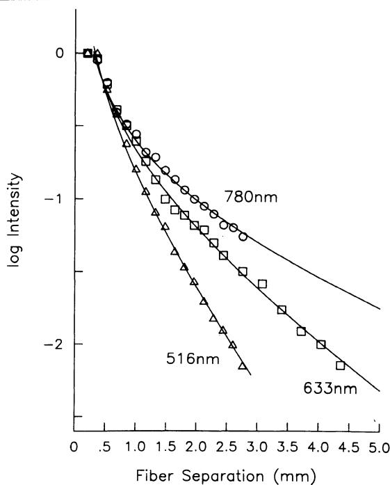
**Figure 2-11.** Emission intensity measurements for light diffusing within human forearm skin, as a function of probe separation. The solid lines are least-squares fits to the data by equation 2.36. (Reproduced from [18].)
