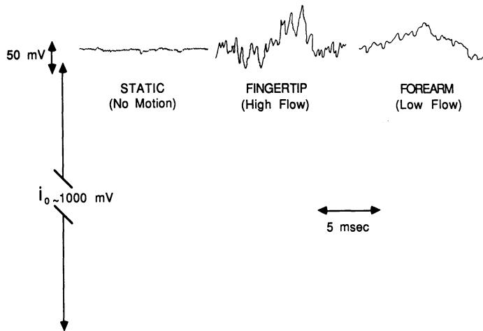
**Figure 2-6.** Schematic of typical signal detected with a laser-Doppler flowmeter. Phototube current  $i(t)$  versus time. The DC (average) component is designated as  $\langle i \rangle_{dc}$ , so  $i_{sc}(t) \equiv i(t) - \langle i \rangle_{dc}$ .
