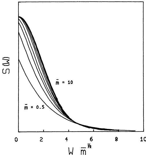
**Figure 2-5.** Normalized spectra, showing the effect of multiple scattering (different values of  $\bar{m}$ ). Curves are plotted as a function of the reduced variable defined in equation 2.19.
