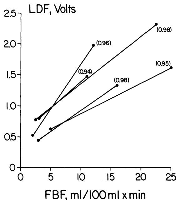
**Figure 8-3.** LDF-FBF relationship from five separate studies. Lines are drawn over the individual ranges of blood flow. Correlation coefficient for each study is indicated. Although there was a highly linear relationship for each study, slopes and intercepts varied considerably among separate studies. (From [1], by permission.)
