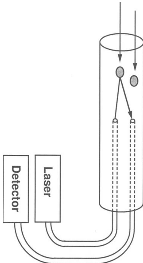
**Figure 1–4.** Catheter laser-Doppler velocimeter. For details see chapter 7.
