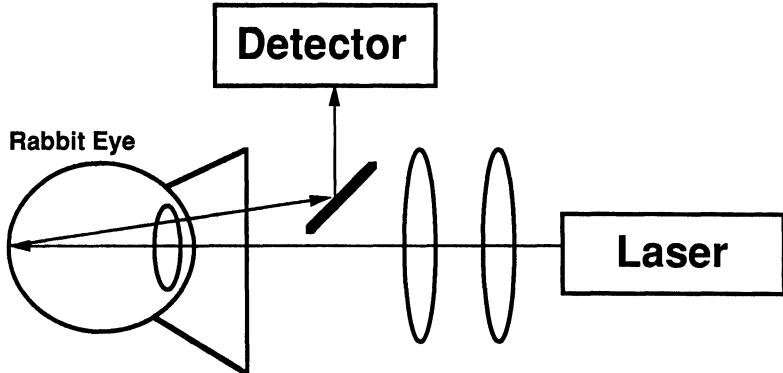
**Figure 1–3.** Retinal laser-Doppler velocimeter. For details see chapter 19.
