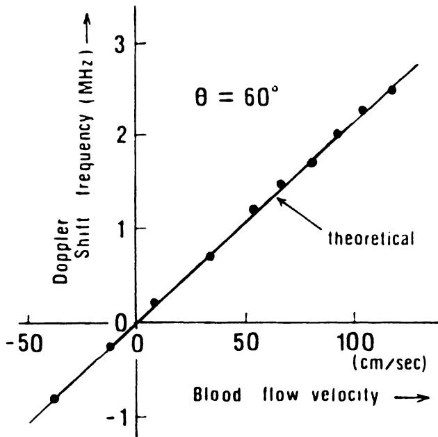
**Figure 7-3.** Linear relationship between velocity obtained from maximum Doppler frequency and free-stream flow velocity when a bare fiber is inserted into the flow at a  $60^\circ$  angle, avoiding the wake produced by a catheter. Directional Doppler shifts were obtained by a frequency-shift heterodyne method. (From Nishihara et al. [4], figure 8.)
