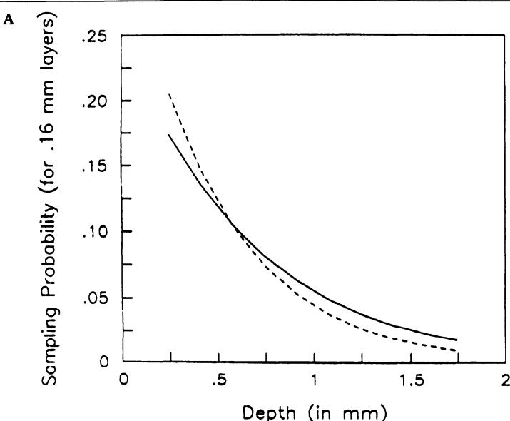
**Figure 2-12.** Relative probabilities of sampling different layers in human skin, using a laser-Doppler probe consisting of two 0.1 mm fibers separated by 0.5 mm. A. Depth distribution. B. Probability distribution of sampling at a distance perpendicular to the plane defined by the fiber pair. Solid line: 785 nm. Dotted line: 632 nm.
