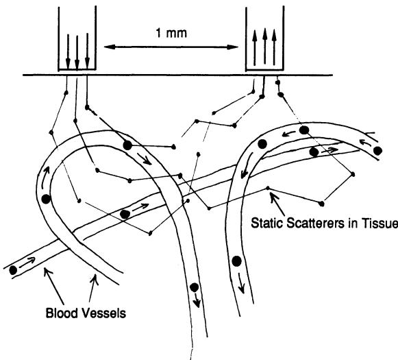
**Figure 2–2.** Schematic diagram of light diffusing through vascularized tissue.
