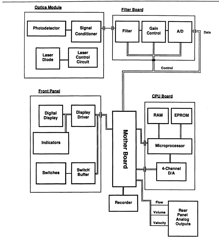
Figure 5–5. Block diagram of Laserflo Blood Perfusion Monitor.
