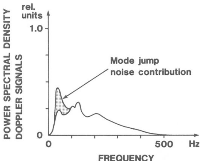
**Figure 6-13.** Power spectral density of laser-Doppler signals from forearm blood flow with and without thermal stabilization. Each spectral density curve is an average of 200 recordings. Thermal stabilization of the laser cavity eliminated the noise from mode jumps in the low-frequency part of the spectrum. (From [14] with permission from the International Federation for Medical and Biological Engineering.)
