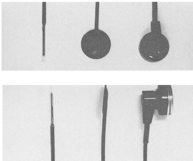
**Figure 3–4.** Probes for both the LD-5000 and LD-6000 systems. Pictured from left to right are the needle, flat, and standard probes seen from above (top) and from the side (below).
