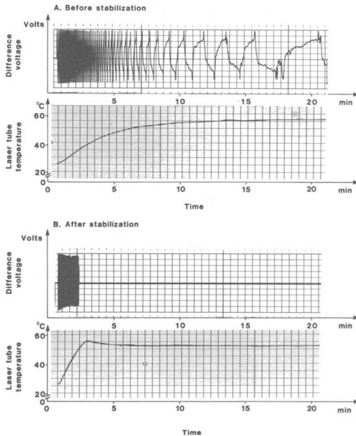
**Figure 6-12.** Laser performance before (A) and after (B) thermal stabilization of the laser tube. After the initial heating period (B), the closed-loop control of the laser thermal stability completely eliminated the mode-jump noise. (From [14] with permission from the International Federation for Medical and Biological Engineering.)
