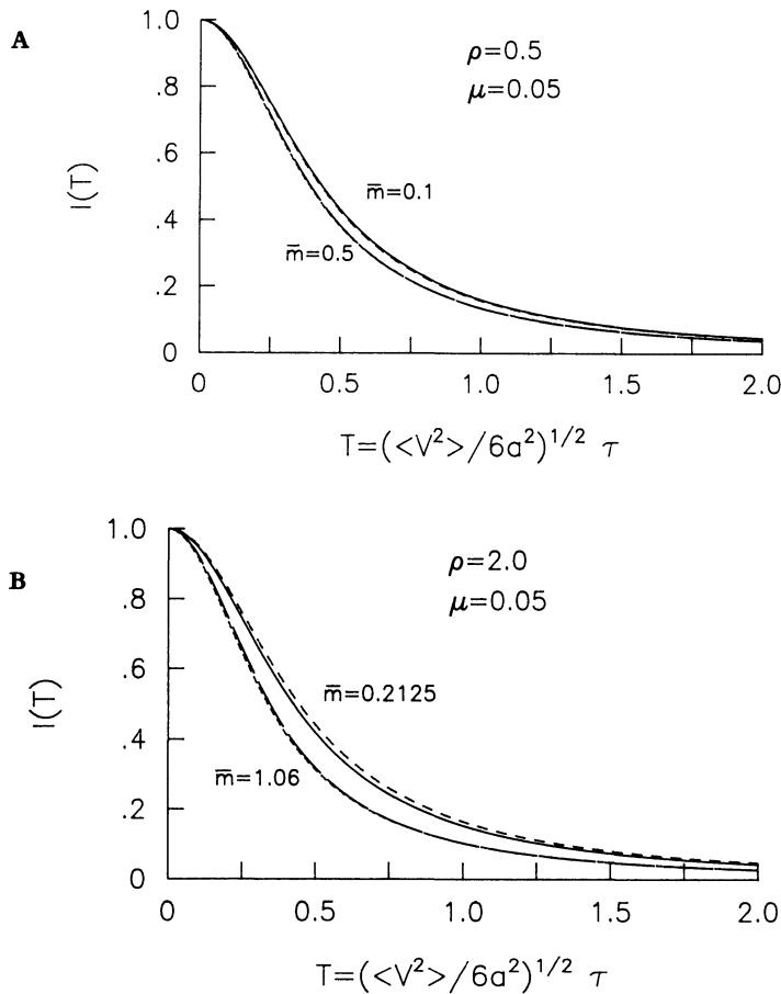
**Figure 2-8.** Photon autocorrelation functions calculated according to equations 2.15 and 2.29, plotted as a function of the reduced time variable  $T = \frac{\langle V^2 \rangle^{1/2} \tau}{\sqrt{6a}}$ . Absorption,  $\mu = 0.05$ .
