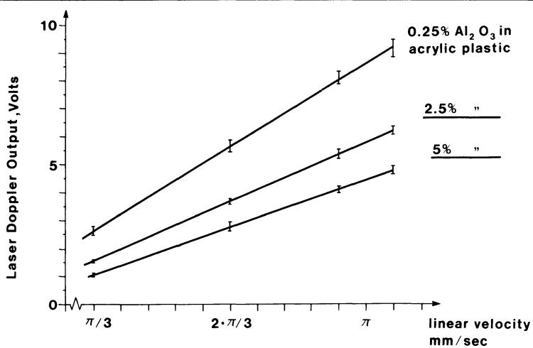
**Figure 6-8.** The relation between the linear velocity of a rotating disk manufactured from moulded acrylic plastic and laser-Doppler output voltage. Observe the strong influence of the concentration of the scatterers in the moulded disk. (Öberg, Petersson and Rohman, unpublished results.)
