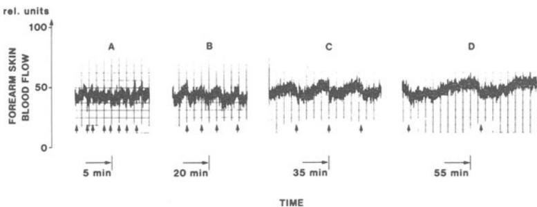
**Figure 6-10.** Recording of forearm skin blood flow. The blood flow signal mixed with noise from an unstabilized laser-Doppler instrument (Perimed PF1d). The mode jumps occurred at the moments indicated by arrows. The periodicity of the noise varies with the temperature of the laser cavity. This type of noise can easily be misinterpreted as vasomotion. (From [14] with permission from the International Federation for Medical and Biological Engineering.)
