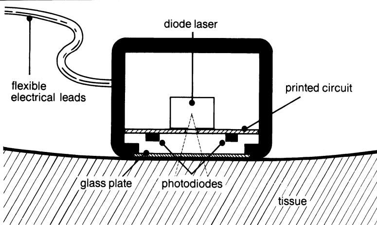
**Figure 6-3.** Minilaser-Doppler flow monitor without optical fibers. The laser diode is mounted in between the two receiving photodiodes in a housing that is attached directly to the tissue surface under study. (From [5] and [6] with permission from the American Institute of Physics.)
