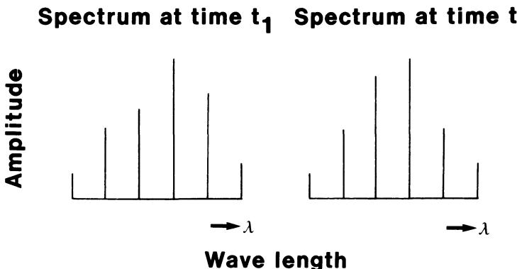
**Figure 6-9.** Longitudinal mode frequency distribution from a He-Ne laser on two occasions  $t_1$  and  $t_2$ . Mode-jump noise occurs when the total energy of the laser is redistributed among the different modes that can exist in the laser cavity.
