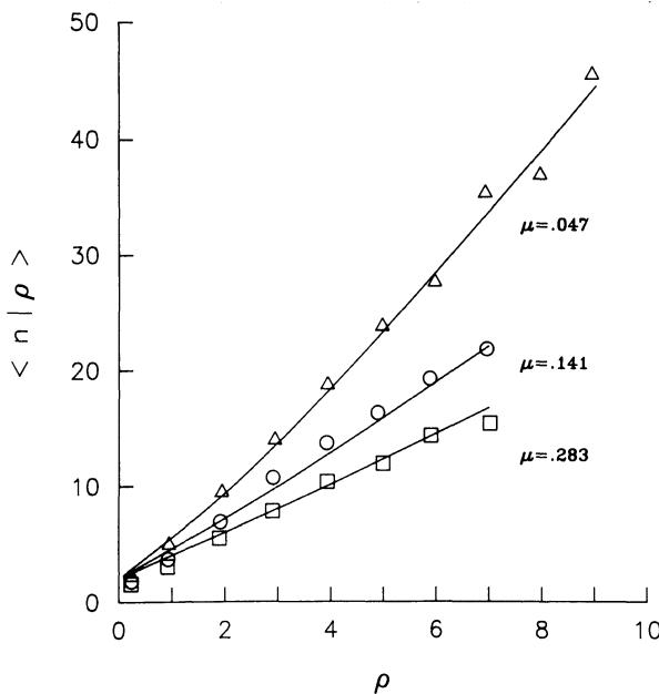
**Figure 2–10.** The variation of pathlength with probe separation, calculated according to equation 2.31 and compared with Monte-Carlo calculations performed for an isotropic continuum. (Reproduced from [18].)
