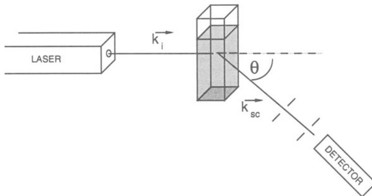
**Figure 2–1.** Schematic of spectrometer used for performing dynamic light-scattering measurements.
