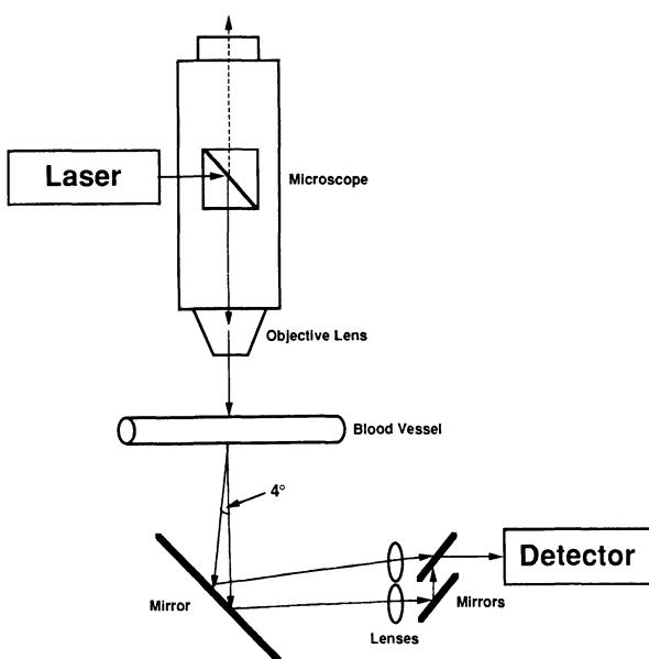
**Figure 1–2.** Laser-Doppler microscope for measuring red blood cell velocity in a single microscopic blood vessel.
