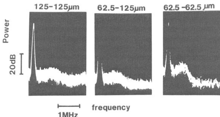
**Figure 7-6.** Doppler spectra obtained from a dual-fiber heterodyne system for three different fiber spacings, achieved by using pairs of side-by-side fibers of either 125  $\mu\text{m}$  or 62.5  $\mu\text{m}$  outer diameters. The sharp peak at left is the zero Doppler shift point. The broad peaks are the Doppler spectra due to blood flow. (From Kajiya et al. [7], figure 3.)
