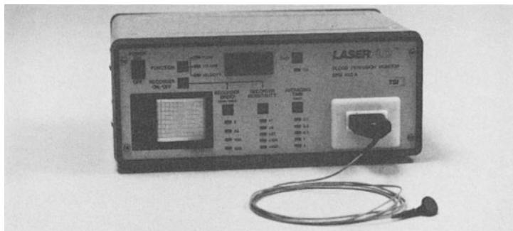
**Figure 5–1.** The Laserflo Blood Perfusion Monitor.
