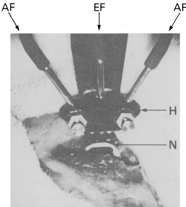
**Figure 15–7.** Arrangement of LDF probe for measuring blood flow of sciatic nerve in rat. EF, efferent optical fiber; AF, afferent optical fiber; H, nerve holder; N, sciatic nerve. (Reproduced from Rundquist et al. [60], with permission.)
