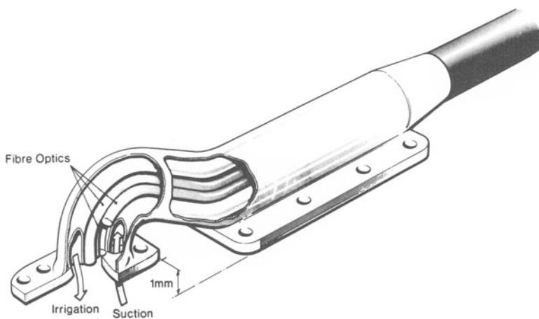
**Figure 10-6.** LDF flow probe designed for intra-oral or buried use. (Reprinted with permission from [15].)
