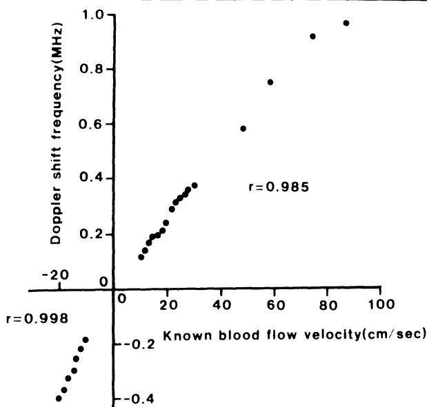
**Figure 7-7.** Relation between free-stream flow velocity and the Doppler shift frequency at the spectral peak for a dual-fiber system with center-to-center spacing of 62  $\mu\text{m}$ . (From Kajiya et al. [7], figure 5.)
