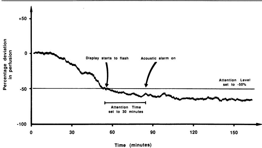
**Figure 4-4.** Monitoring successive impairment in skin-flap blood flow by the Periflux PF3 laser-Doppler perfusion monitor.
