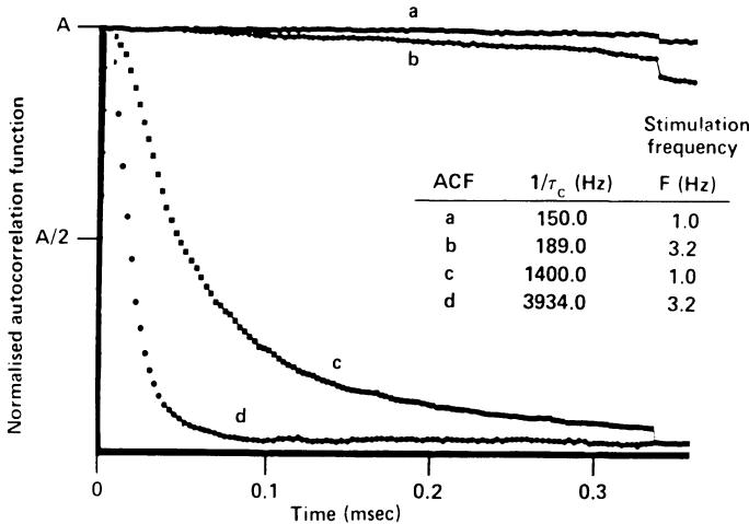
**Figure 6-1.** Autocorrelation functions (ACF) obtained from the intensity fluctuations produced by manipulated optical fibers: (a) and (b) are from 50  $\mu\text{m}$  core graded-index fiber, and (c) and (d) are from Periflux 763  $\mu\text{m}$  core step-index fibers. The stimulation and mean intensity fluctuation frequencies are tabulated. (From [3] with permission of the International Federation for Medical and Biological Engineering.)
