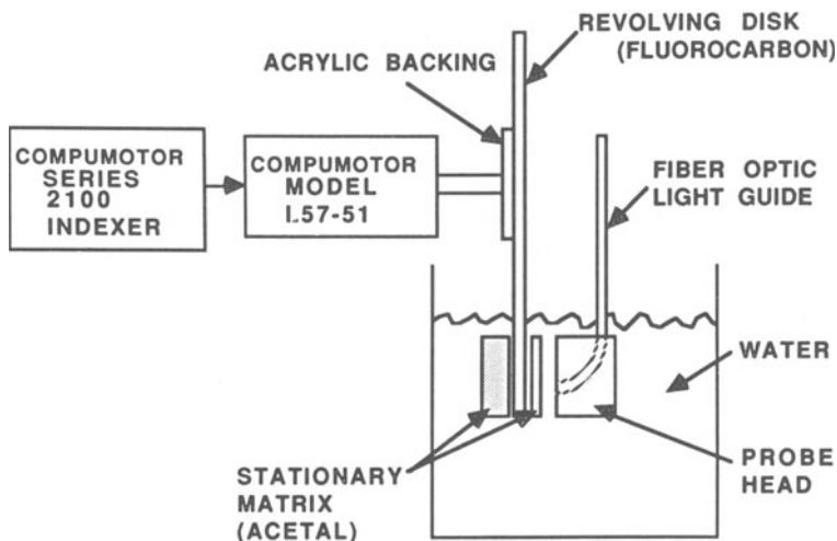
**Figure 6-7.** Model to simulate perfused tissue. Revolving fluorocarbon disk produced Doppler shifts in light scattered back to fiber optic light guide. Acetal block simulated light scattering by static tissue. Optical fibers delivered light to and carried scattered light back from rotating disk. For clarity, only one fiber is shown. A stepping motor controlled disk velocity precisely. (From [7] with permission from the American Physiological Society.).
