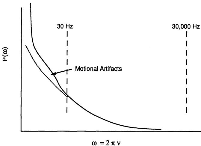
**Figure 2–7.** Schematic representation of the power spectrum of the detected photocurrent, showing 30 Hz and 30,000 Hz cutoffs.
