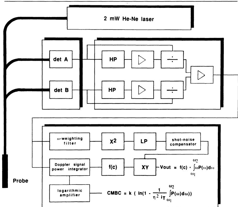
**Figure 4-1.** Schematic diagram of the basic operating principle of Periflux PF2b and PF3 (for definition of symbols, see equations 4.1 and 4.2 in the text).
