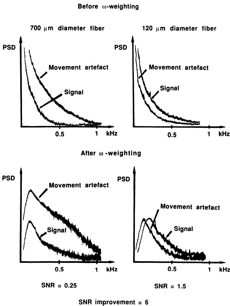
**Figure 4-2.** Power spectral density (PSD) before and after  $\omega$ -weighting caused by fiber-movement artifacts and blood flow, respectively, as recorded by laser-Doppler flowmeters equipped with 700  $\mu\text{m}$  and 120  $\mu\text{m}$  step-index fibers. SNR = signal-to-noise ratio.
