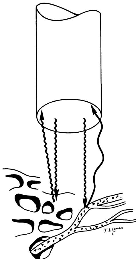
**Figure 17–3.** Incident light and backscattered, frequency-shifted light are transmitted through one optical fiber.
