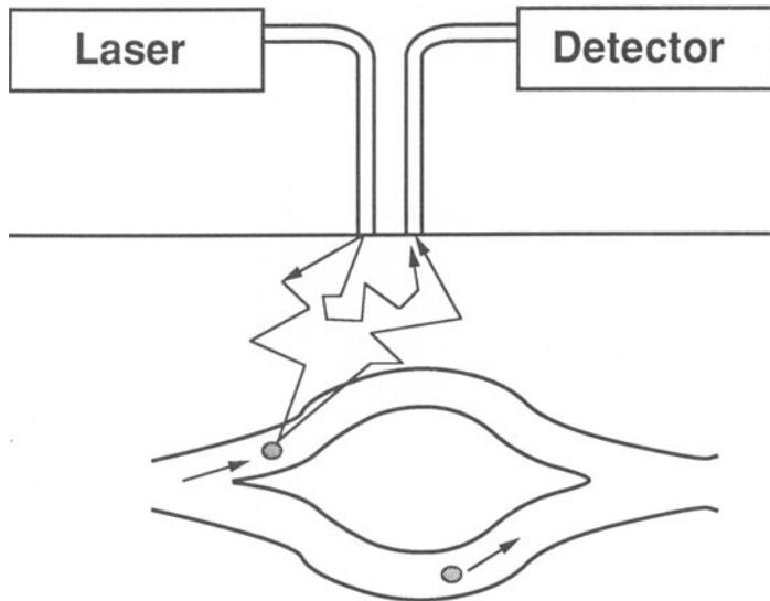
**Figure 1–1.** Laser-Doppler measurement of tissue perfusion. Laser light is typically delivered to tissue and returned to a detector by fiber optic light guides. Light in tissue is diffusely scattered by stationary tissue. Such light reaches the detector without being Doppler-shifted. Photons that encounter moving red blood cells experience a Doppler shift.
