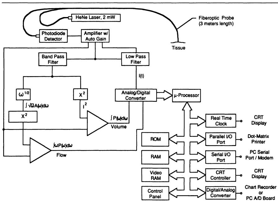
**Figure 3-3.** Block diagram of the LD-6000 system.
