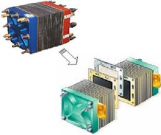
Figure 1. A PEM fuel cell stack
