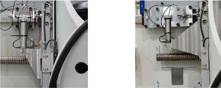
Figure 7. Comparison of the original (left) and the revised (right) actuator coupling configuration
