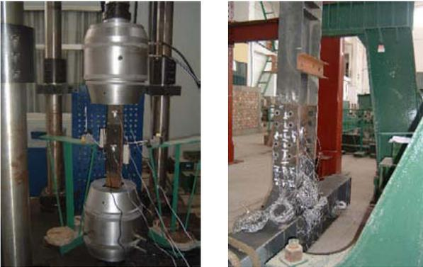
(a) Friction component test                      (b) T-shaped joint test
