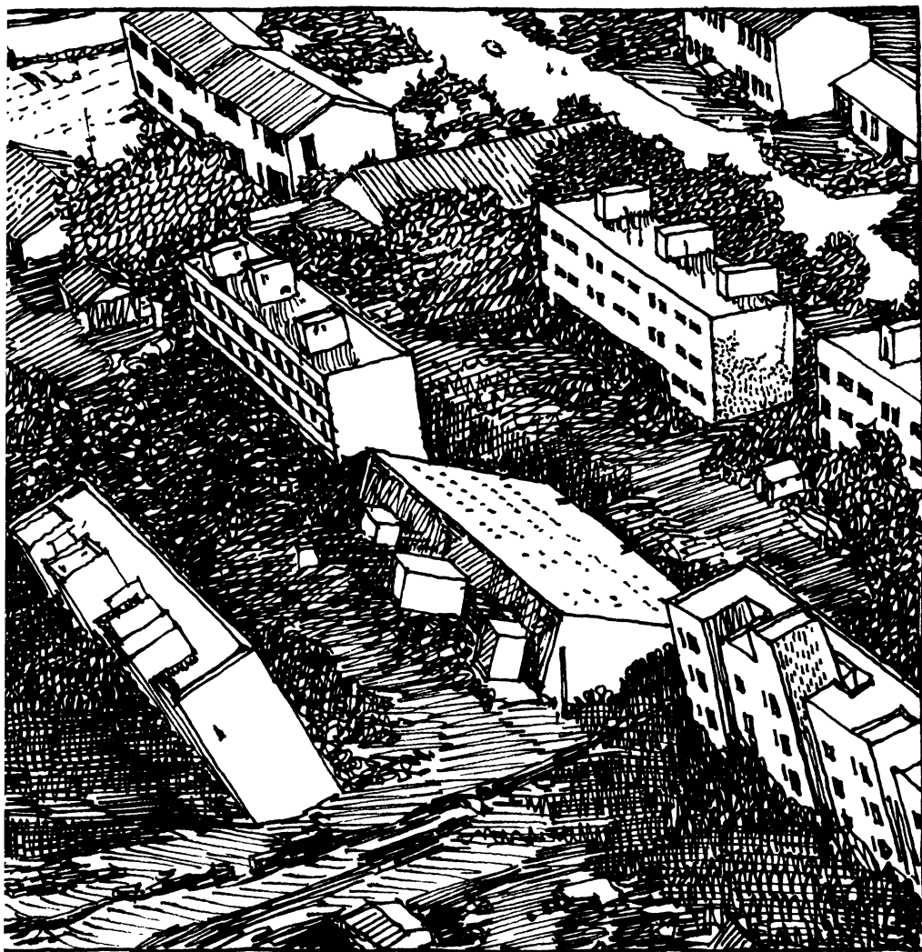
6.6 Niigata Apartment Buildings: After the Earthquake
