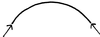
3.13b Dome Reactions —Shallow Sphere
