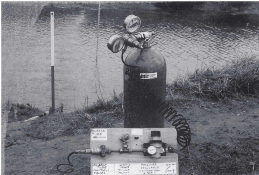
Figure 4.4 The equipment used in the integrating rising air float technique.
