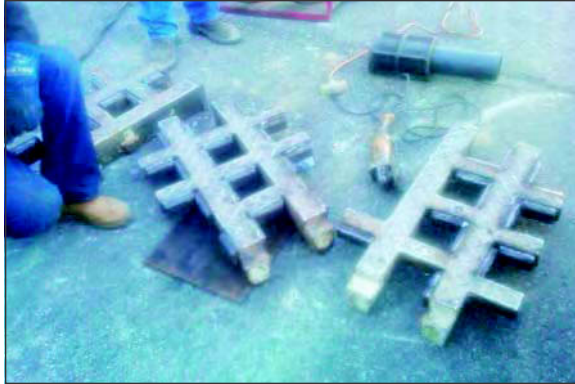
Figure 9. Crusher grill plate modifications
