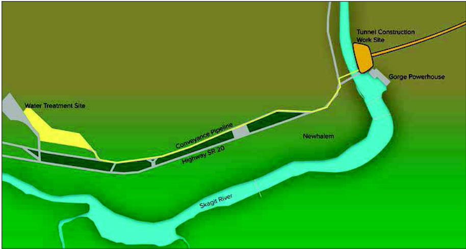
Figure 2. Water management layout
