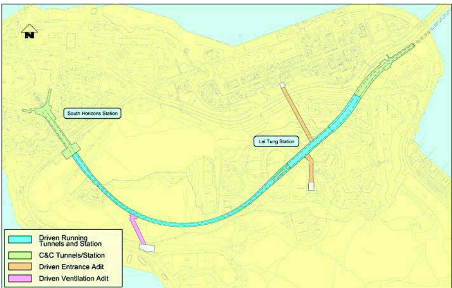
Figure 3. Plan of Contract 904 tunnels
