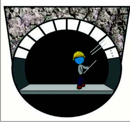
Figure 8.1. A worker loads slats into the McNally Pockets
