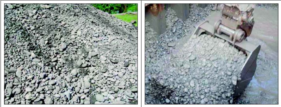
Figure 4. Left: Springfield Intake Facility. Gravel and cobbles excavated from the launch shaft. Right: Gravel and cobbles excavated from the rescue shaft. (Del Nero 2008)
