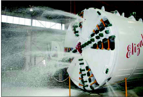
Figure 3. Demonstration of foam injection from TBM cutterhead injection ports
