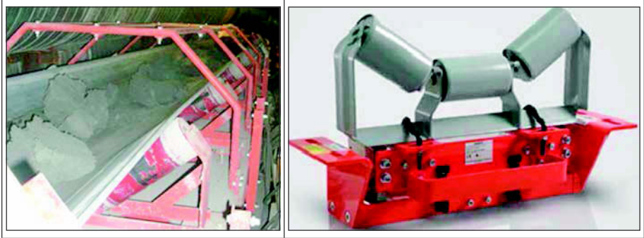
Figure 3. Belt scale on the TBM conveyor and the Siemens Milltronics belt scale unit
