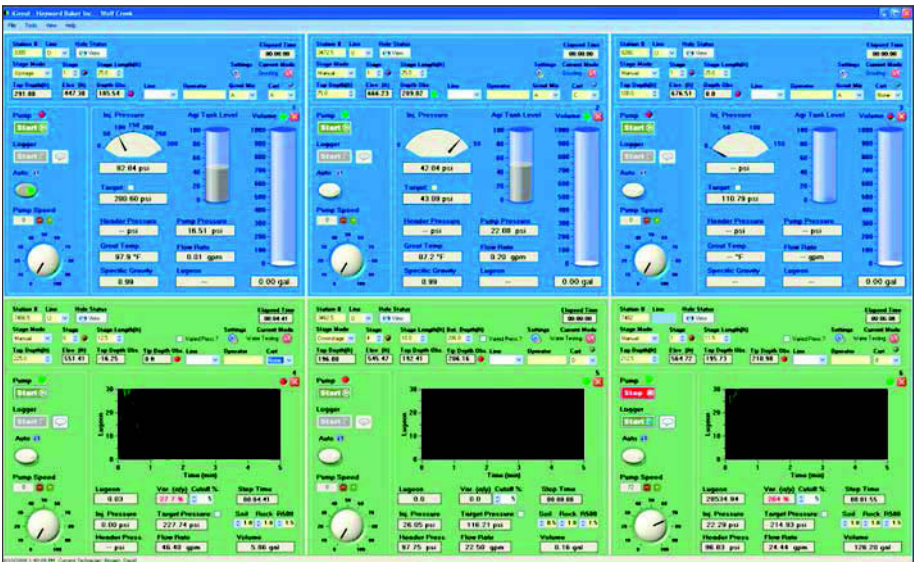
Figure 8. Example of iGrout control screen for water testing and grouting operations
