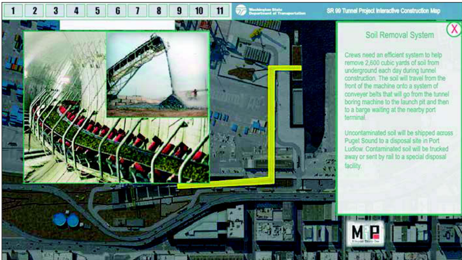
Figure 8. Conveyor route at SR99 tunnel (Source: Washington State Department of Transportation)
