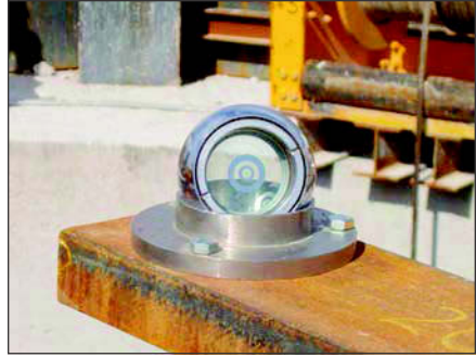
Figure 9. Taylor Hobson spheres used for transferring survey control through the North Kenmore Portal (shaft)
