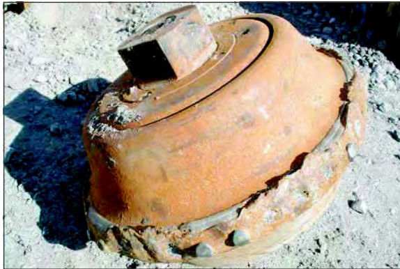
Figure 14. Damaged cutter—first 20ft of yard lead tunnel
