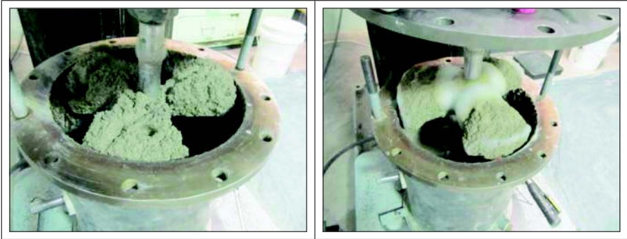
Figure 7. (a) 15% W silica sand sample conditioned with 3% concentration ABR 5, 25% FIR, and FER of 17; (b) 15% W silica sand sample conditioned with 3% concentration Meyco SLF 47, 25% FIR, and 17% FER after 30 minutes of test
