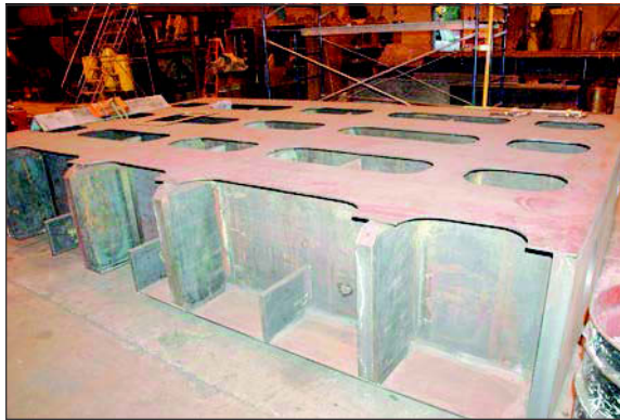
Figure 8. Gate fabrication in progress
