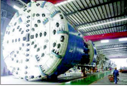
Figure 2. Shop assembly of the main beam TBMs
