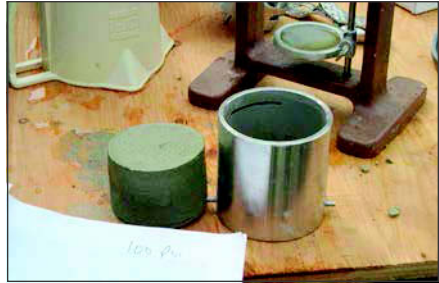
Figure 3. A sample of the non-cementitious grout field-tested before the trial program. Note the decreased volume of the sample due to intended pressure filtration.
