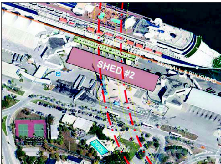
Figure 4. TBM orientation to existing structures on north shore of Dodge Island
