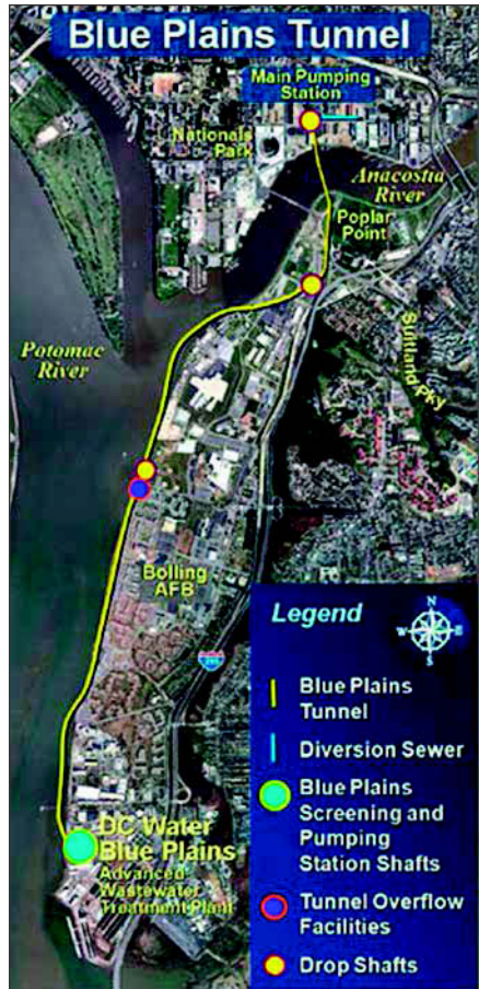
Figure 1. Blue Plains tunnel alignment
