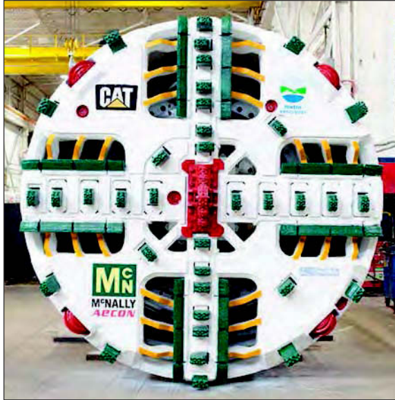
Modification to cutterhead design to reduce mitigate the need for intervention
