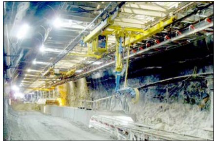
Figure 16. RPHT—Shotcrete manipulator with swiveling and telescopic spraying arm, covering a working area of 12 meters in length and a 210^\circ sector (Courtesy of Rowa, www.rowa-ag.ch )
