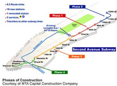
Figure 1. MTA's general arrangement route plan for the Second Avenue Subway in Manhattan, New York City
