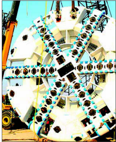
Figure 4. Mixed ground cutterhead for the Lot 1 machine
