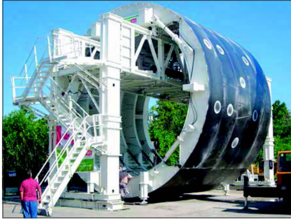
Figure 4. Tunnel form inspection
