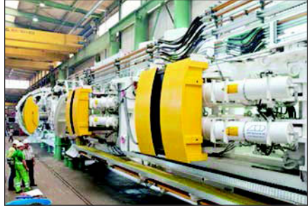
Figure 5. Additional gripping systems behind the TBM
