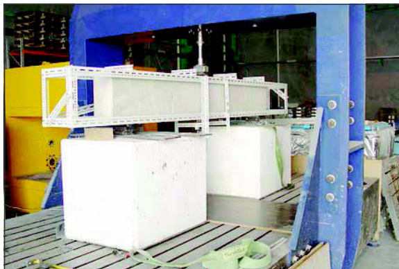
Figure 5. Bending test on FRGC beams
