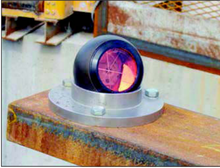
Figure 8. Bæchler prisms used for transferring survey control through the North Kenmore Portal (shaft)
