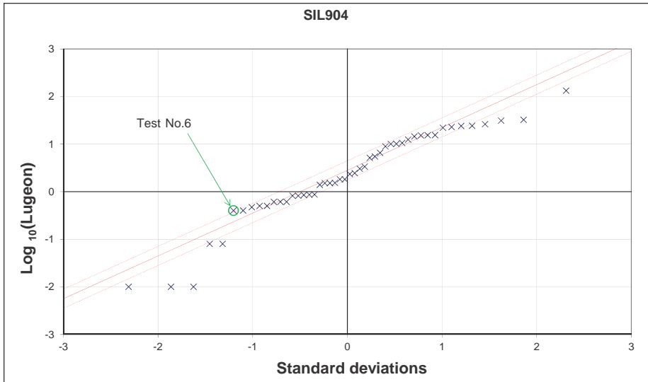
Figure 4. Plot of packer test data set from Contract 904, using the procedure of Raymer (2001, 2005)
