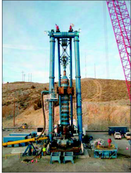
Figure 1. Blind bore machine
