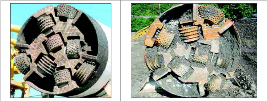
Figure 5. Springfield Intake Facility. Left: Soltau RVS 600AS MTBM prior to launch. Right: MTBM after recovery from rescue shaft. (Del Nero 2008)
