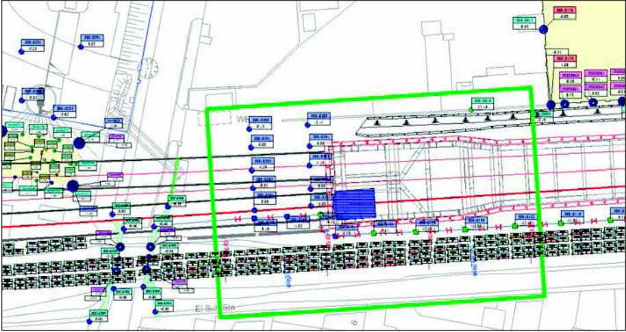
Figure 5. TBM operators view of surface data alongside the automatic zone of influence indicator
