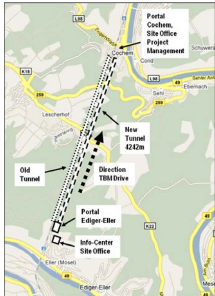
Figure 4. Schematic view of the existing tunnel (first tube) and the new tunnel (second tube) (Source: ABT, 2012b based on Google Maps)
