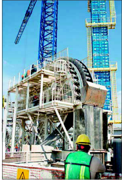
Figure 6. Vertical belt conveyor with vertical belt cassette in the background (tower on the right)
