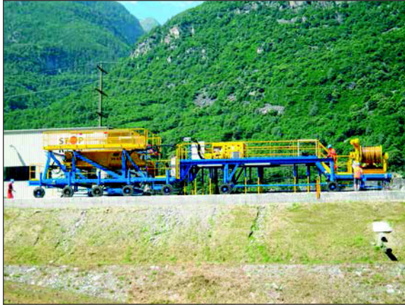
Figure 6. Self-propelled concrete transport shuttle (Source: ABH, 2010)
