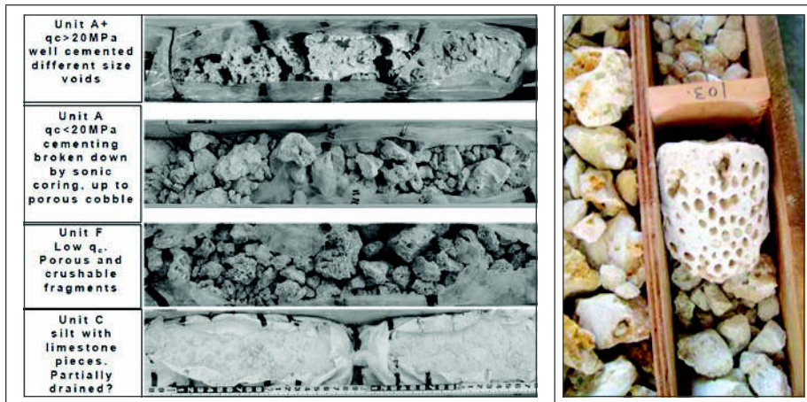
Figure 4. Sonic cores of different units of Key Largo limestone in Layer S7 identified on the basis of CPT profiles
