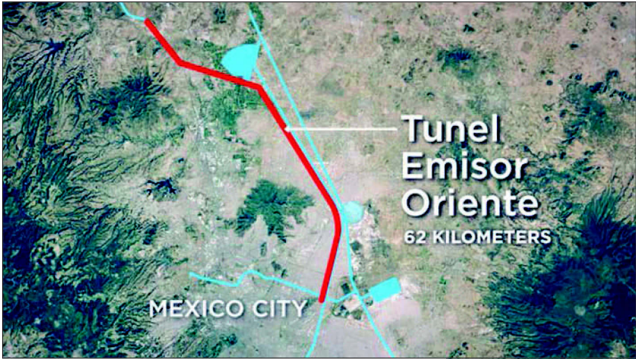
Figure 1. Layout of the Emisor Oriente wastewater tunnel
