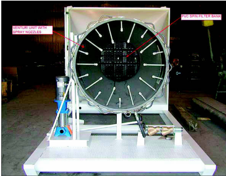
Figure 6. End view of wet scrubber system showing venturi unit with spray nozzles and PVC spin filter bank
