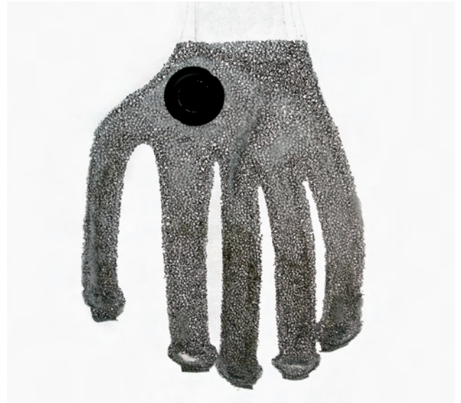
WELDED FOAM. Sandwiched between two layers of plastic film, a foam sheet is RF welded to make a bladder insert for a sports glove. Working as a spacer, the foam keeps the plastic sheets apart.
