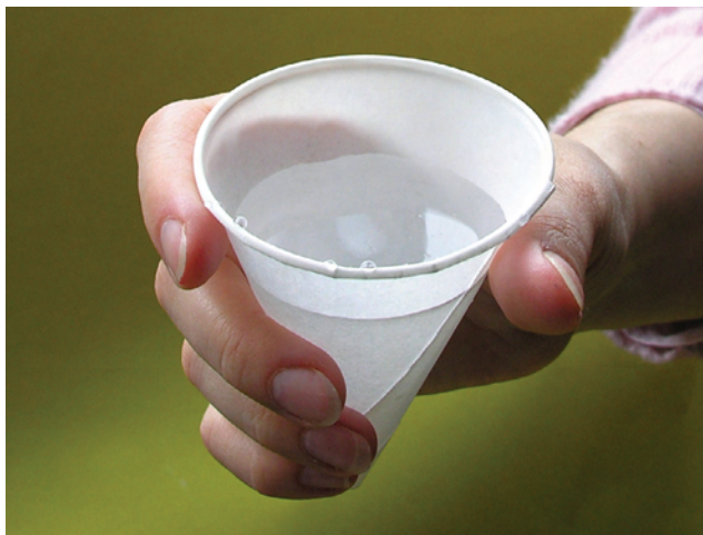
WAXED. Paper absorbs water, but it can be waterproofed with wax.
