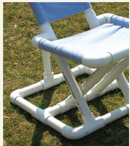
PVC CONNECTORS make turning corners easy. The designer connected the structures with PVC solvent cement, available in any hardware store. Design: Whitney Wright, MICA.
