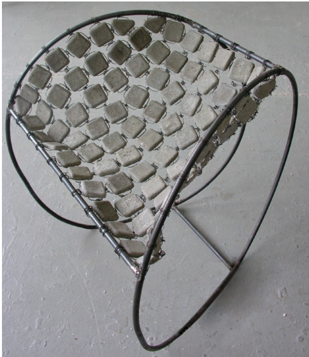
FLEXIBLE CONCRETE. The seat of this chair is made of linked concrete blocks. Each block was cast with wire “ears.” After the concrete cured, the blocks were connected with wires to create a comfortable seat suspended on a steel frame. Design: Kwok Pan Fung, MICA.
