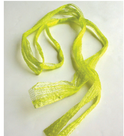
POLY IKAT TAPE is a strong, flexible material from Japan designed for use in resist dying (like tie-dyeing). It splits easily into strips as small as 1/16-inch wide. It has many potential uses, such as weaving a minimal net to carry large objects.
