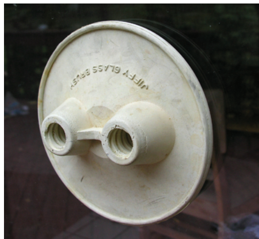
HUGE SUCTION CUP. This special holder used for carrying plate glass uses the principle of the suction cup. Rubber is flexible, and when it is pulled away from the surface, it creates a vacuum and grips the glass safely.
