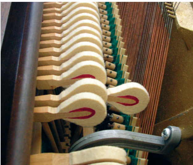
FELT EQUIPMENT. Piano hammers are made from thick sheets of lambswool felt that are shaped and attached to a wooden base. The relative hardness of a piano hammer influences the resulting piano sound.
