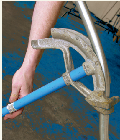
CONDUIT BENDING TOOL is an easy way to shape metal tubes, including steel pipes.
