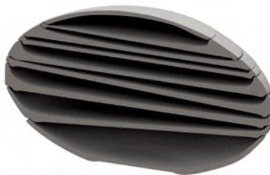
UNIFIED AND UNIQUE. Lollie plates were designed using 3D modeling software and rapid prototyping tools. The final design could be executed in melamine. A section of a computer-generated model helps the designer to see how each plate stacks.
