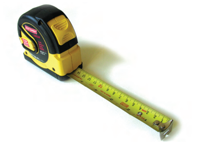
SELF-RETRACTING TAPE MEASURE employs a curved metallic ribbon that remains stiff and straight when extended, but retracts into a coil for convenient storage.
