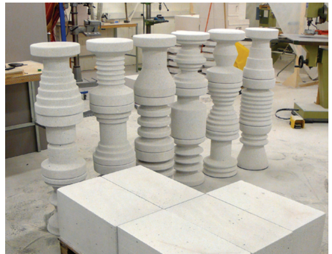
FOAMED CONCRETE contains air bubbles in a cell-like structure, making it five times lighter than ordinary concrete. It can be easily machined into new shapes. Made from an autoclaved cellular concrete block, these stools were turned on a lathe using traditional woodworking tools. Design and photo: Max Lamb.
