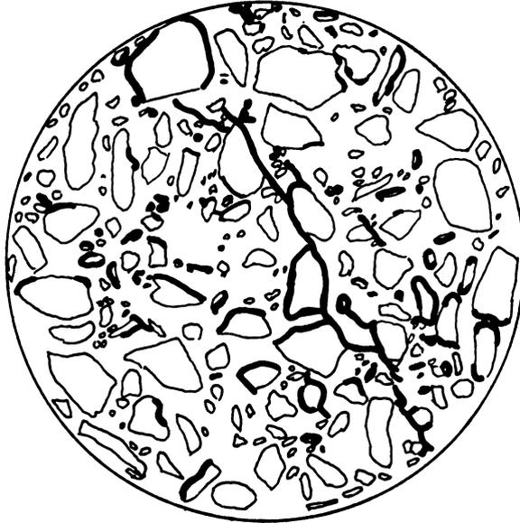
*Figure 8.2 Cracking of concrete due to compressive load (after Hsu and Slate<sup>4</sup>)*
