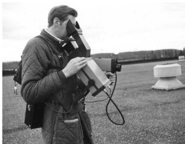
Fig. 58—Surveying a roof with an infrared scanner.
