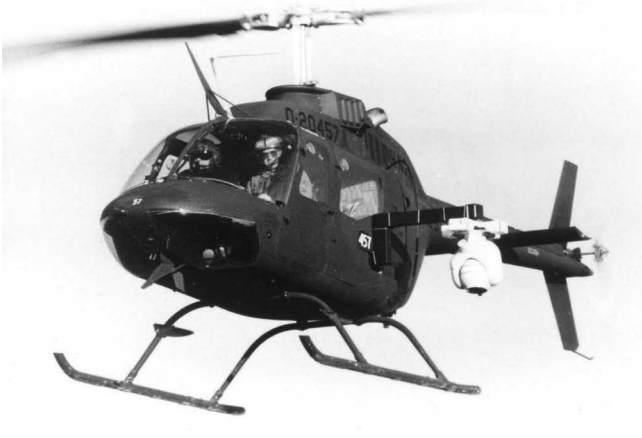
Fig. 60 —Conducting an airborne infrared roof moisture survey from a helicopter.
