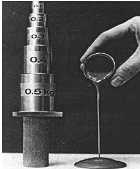
FIGURE 3.25 Quick clay before and after remolding. (Photo courtesy of Haley and Aldrich, Inc.)
