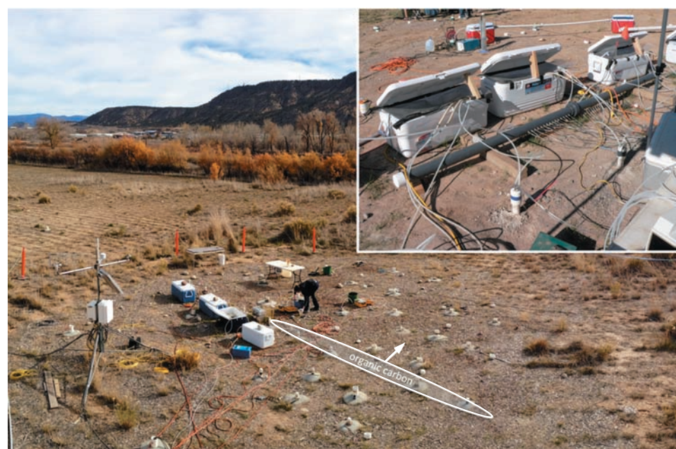
Figure 21.6 Uranium bioremediation. An experimental plot at a United States Department of Energy uranium-contaminated site. Organic carbon (acetate) is being infused into the site (see inset photo) and travels in groundwater in the direction of the arrow shown in the main photo. Acetate is an electron donor for reduction of U^{6+} to U^{4+} , which immobilizes the uranium.
