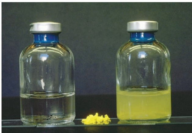
Figure 13.53 Biomining during arsenate reduction by the sulfate-reducing bacterium Desulfotomaculum auripigmentum . Left, appearance of culture bottle after inoculation. Right, following growth for two weeks and biomining of arsenic trisulfide, \text{As}_2\text{S}_3 . Center, synthetic sample of \text{As}_2\text{S}_3 .
