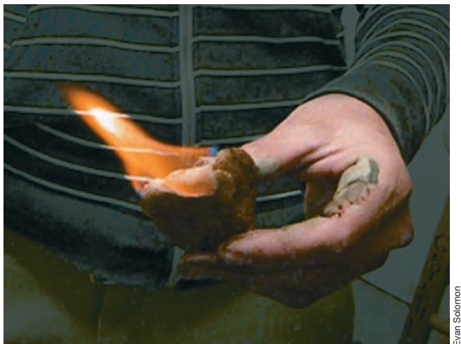
Figure 20.3 Burning methane hydrate. Frozen methane ice retrieved from marine sediments is ignited.
