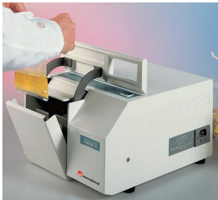
Figure 31.9 A stomacher. Paddles in this specialized blender homogenize the food sample in a sealed and sterile bag. The sample is first suspended in a sterile solution to form a uniform mixture.
