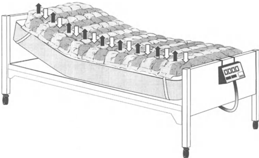
Fig. 6. Alternating air overlay. Adjacent rows of cells ( black and white arrows ) are alternately inflated and deflated to relieve pressure
