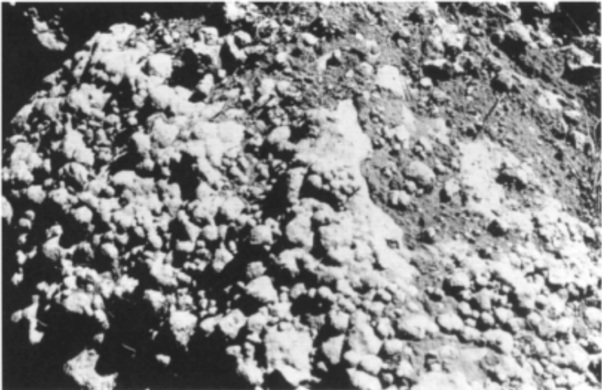
Figure 4.8 Calcrete nodules (10–25 mm diameter) agglomerated into an irregular boulder-sized mass about 1.5 m across, Broken Hill area, New South Wales. (Photo: I.R. Wilson.)
