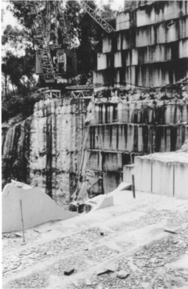
Figure 14.2 Wondabyne sandstone quarry, north of Sydney, New South Wales. Dimension stone quarries have operated intermittently here for over a century, but the worked area covers only 1 ha and is 40 m deep. Note the smooth wire-cut faces and, beneath the crane, presplit blastholes.
