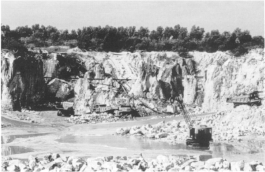
Figure 15.3 Buried karst exposed in a limestone quarry, Kuala Lumpur. This site was formerly a derelict alluvial tin mine, and is being further redeveloped into a housing estate as limestone extraction is completed.
