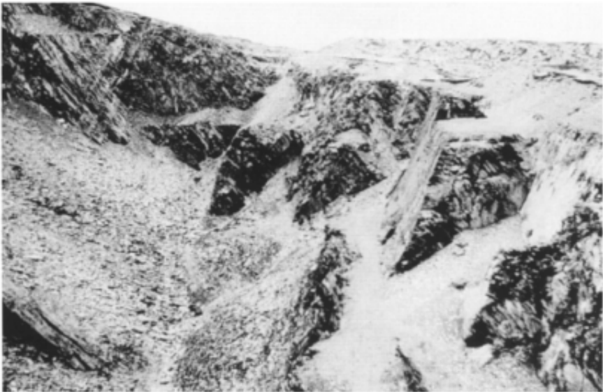
Figure 21.1 Quarry abandonment, old style—a former slate pit in north Wales. Note planar slope failures along a persistent joint set oblique to cleavage and the large proportion of wastage (up to 90% in some slate pits). (Photo: J.H. Whitehead.)
