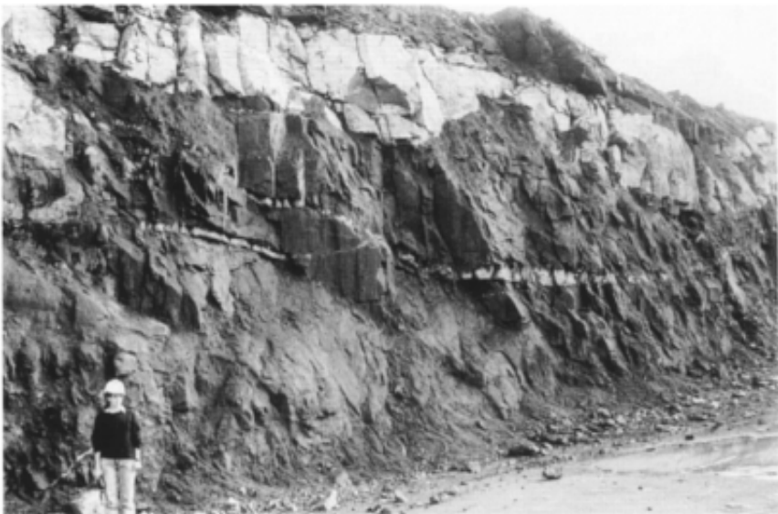
Figure 2.6 Typical bench face at Prospect quarry. The dark rock is olivine-rich picrite, which disintegrates within weeks of exposure, hence the smooth, rounded exposure. The light-coloured rock is better-quality syenitic ‘pegmatite’; note the sharper joint intersections in this more durable material.
