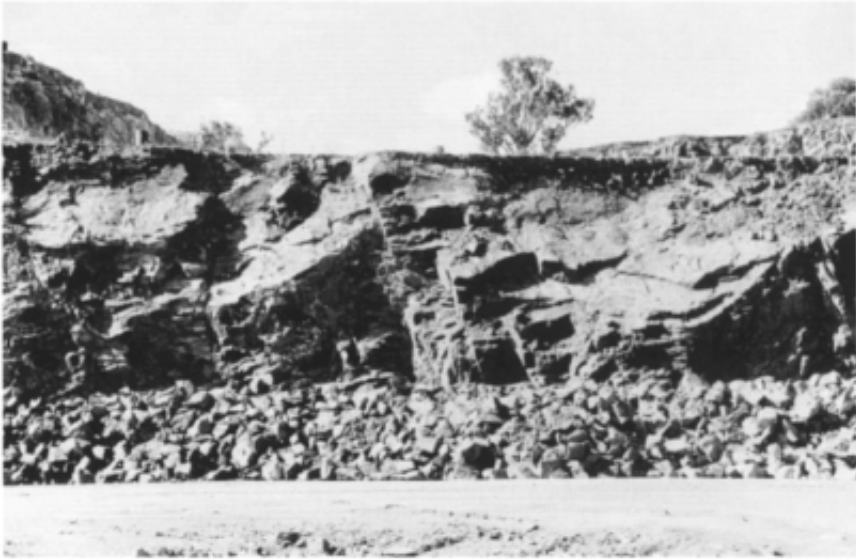
Figure 2.4 Jointed porphyry, Canberra, ACT, Australia. This face is only about 6 m high, but the 40° forward-dipping joints would present a hazard in a higher bench; the joint set dipping at 80° to the right would be a more satisfactory face orientation.
