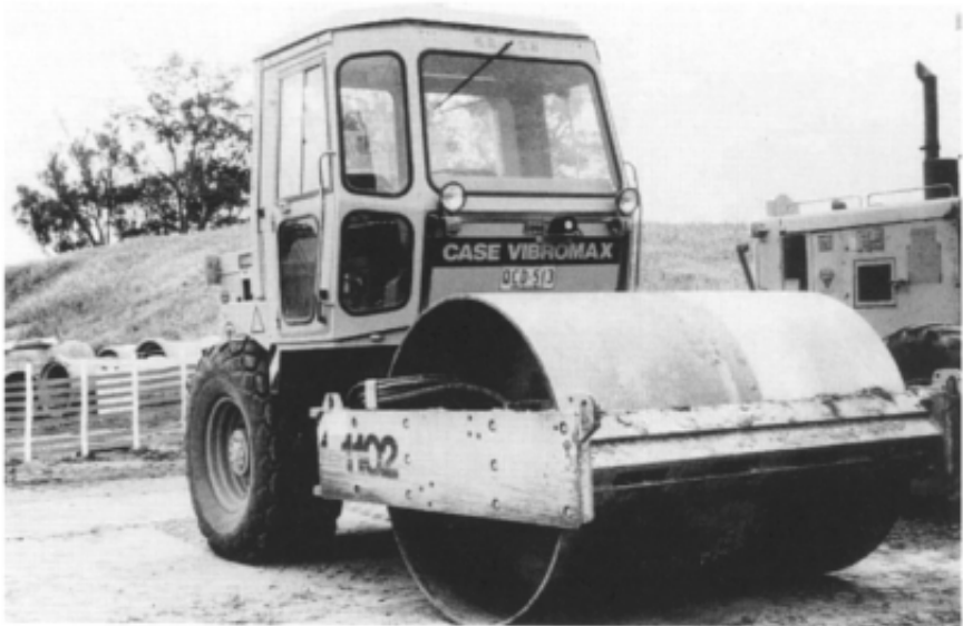
Figure 10.4 Typical vibrating smooth drum roller, mainly used for compaction of granular pavement courses.
