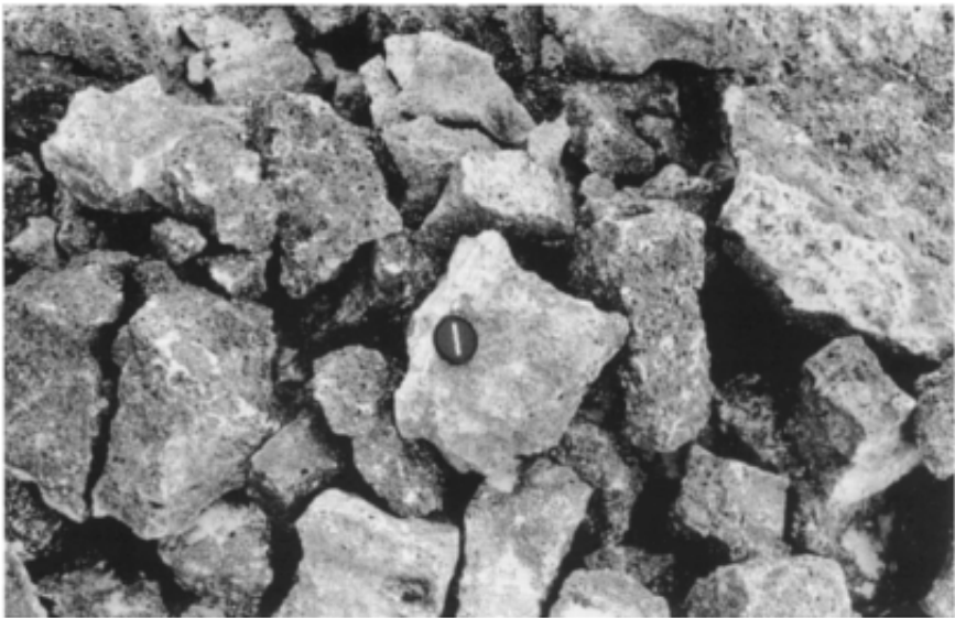
Figure 17.2 Stockpiled rock slag—coarse 'skulls' of cellular blast furnace slag about 0.3 m average size, generally used for open-graded macadam roadbase. A small proportion of fines is generated by on-road rolling, but the strength of these pavements is mainly due to interlocking blocks and self-cementation.
