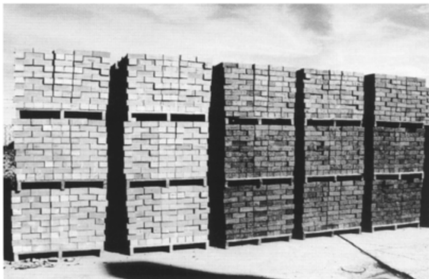
Figure 16.4 Light and dark tones obtained from the same raw materials by changes in kiln ventilation. The actual colours are buff to light brown (left, oxidizing atmosphere) and purple-brown (right, reducing atmosphere).
