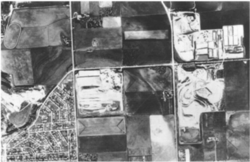
Figure 3.5 Aerial view (about 2 km across) of sand mining south of Adelaide. Note urban encroachment on left and rectangular tailings dams, which occupy half the area of some pits. The sand pit on the far left has since been rehabilitated.
