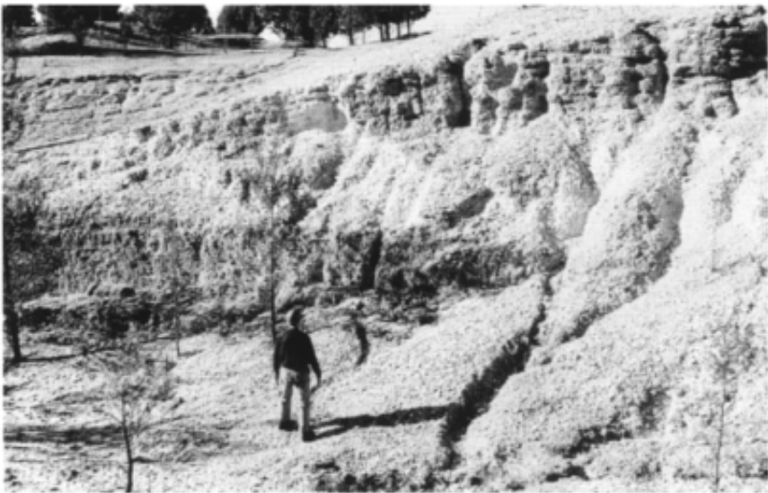
Figure 1.1 Quarry reclamation, the old way. This alluvial gravel pit near Urana, New South Wales, has been simply abandoned. Note that some natural revegetation has occurred, despite a poor soil and gully erosion. On a positive note, this quarry offers a wildlife refuge in an otherwise monotonous farmland plain, and is the only surface exposure of these Late Tertiary gravels in the State.
