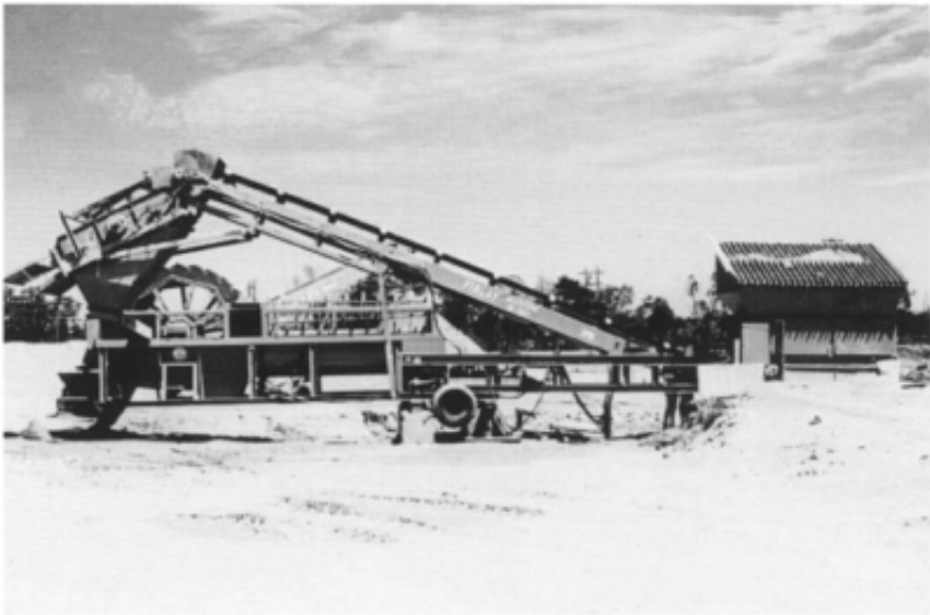
Figure 6.9 Portable sand classification plant, Glenlee, New South Wales. Coarse lumps are shed on the bar screen (at right) and finer clay balls by the vibrating screen (top left). The dry scalped feed is then dropped into a long, narrow, water-filled trough, where it is agitated by a helical screw. Clean coarse sand is lifted out of the trough by the bucketwheel and the fine sand residue is drained away.
