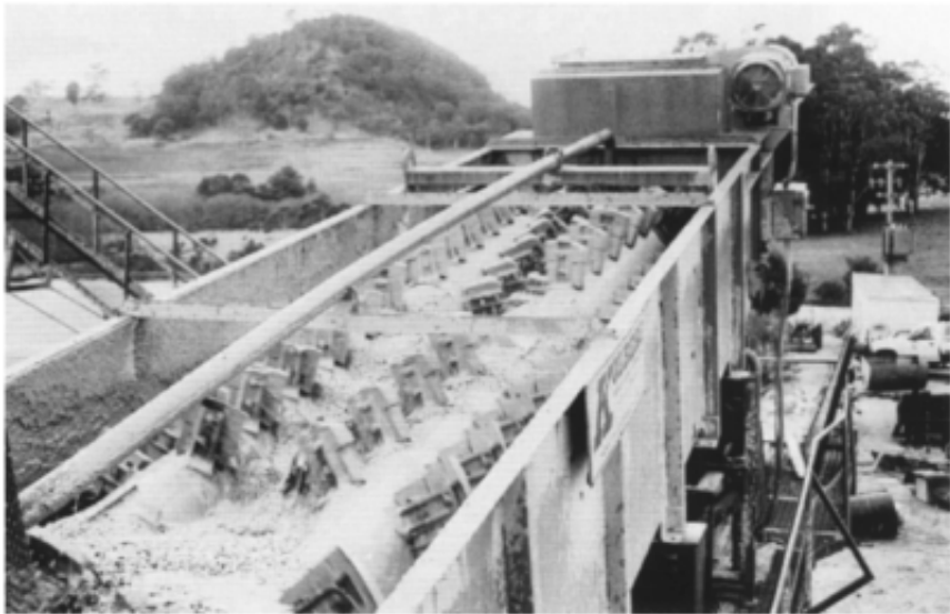
Figure 3.9 Weakly cemented sandstone being disaggregated in a logwasher (note contra-rotating paddles), Kangaloon, New South Wales.
