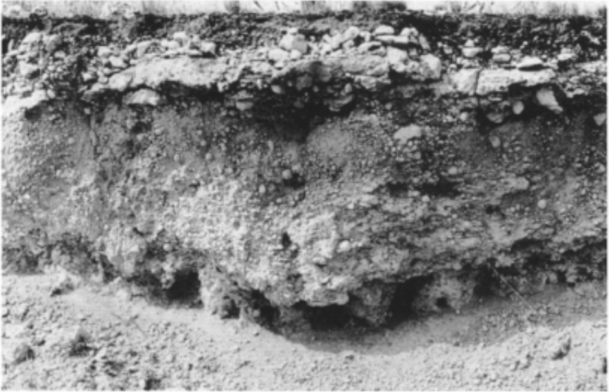
Figure 4.7 Typical calcrete profile about 2.5 m deep in a gravel pit near Mannum, South Australia. Note the well-cemented hardpan at the top, nodular calcrete beneath and loose powder calcrete at base.
