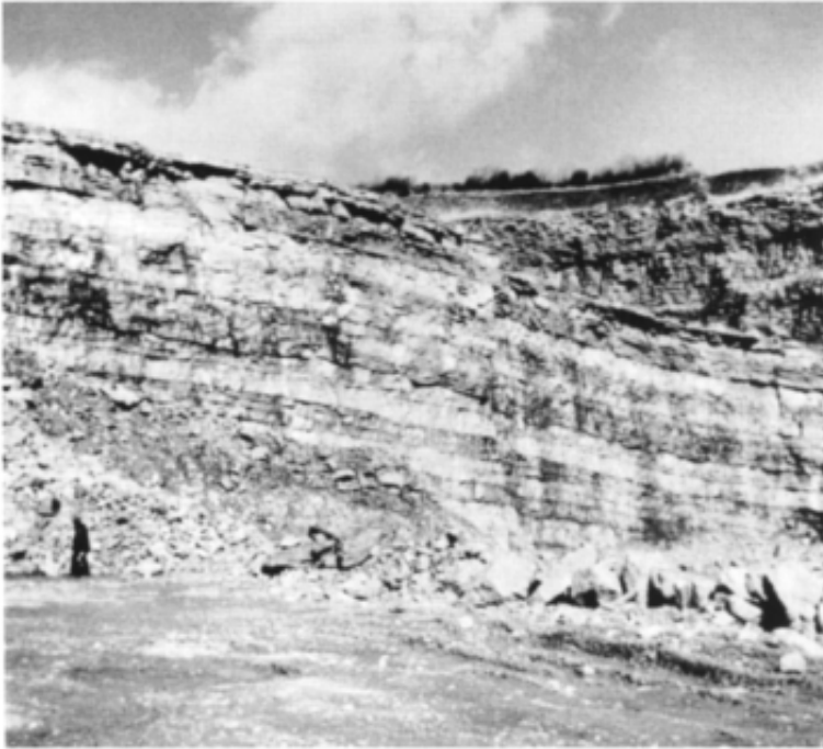
Figure 15.1 Interbedded limestone and shale, naturally proportioned for cement raw material ('cementstone'), Hendry Quarry, North Wales. (Photo: J.H. Whitehead.)
