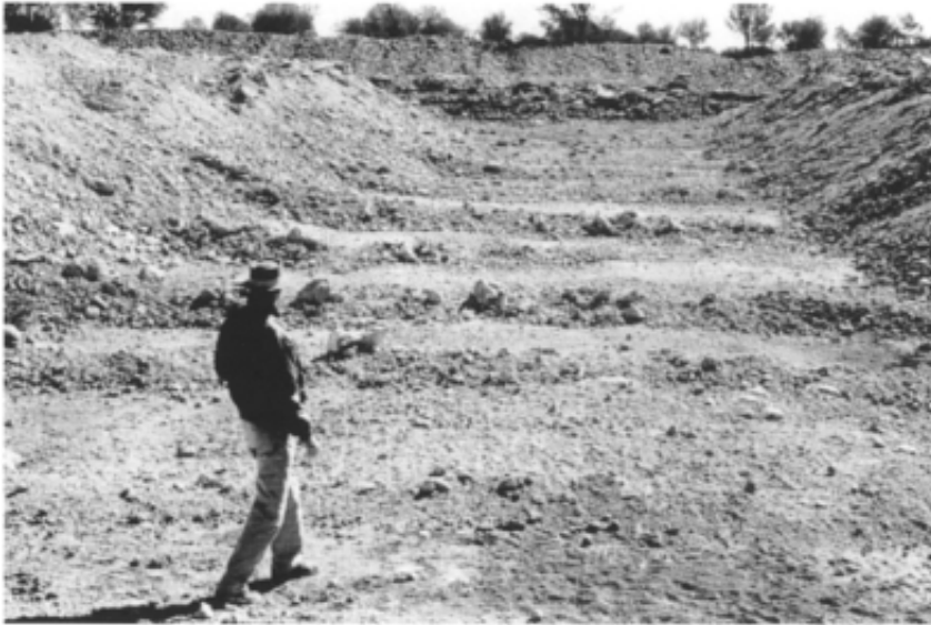
Figure 4.2 Typical road gravel pit, western New South Wales. This scrape is deeper and narrower than most, and overburden has been stockpiled at the edges for site rehabilitation.
