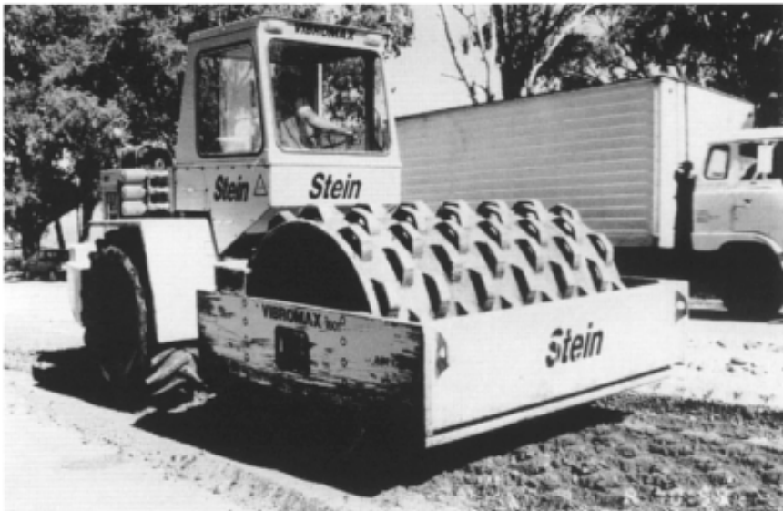
Figure 10.5 Vibrating padfoot roller. Note imprint on soil—this roller is for earthworks compaction, not for finishing or sealing layers.
