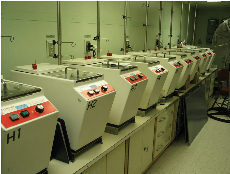
Fig. 1. The line of deglycerolization (washing) machines Haemonetics ACP-115 – first fully automated machines
