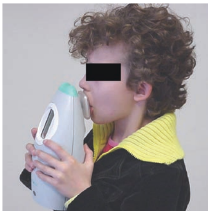
Figure 1. Measurement of FeNO in a child using a hand-held device with an electrochemical sensor. Maintaining a low, constant expiratory flow is facilitated by optical, auditory and visual feedback signals. The result is immediately available.
