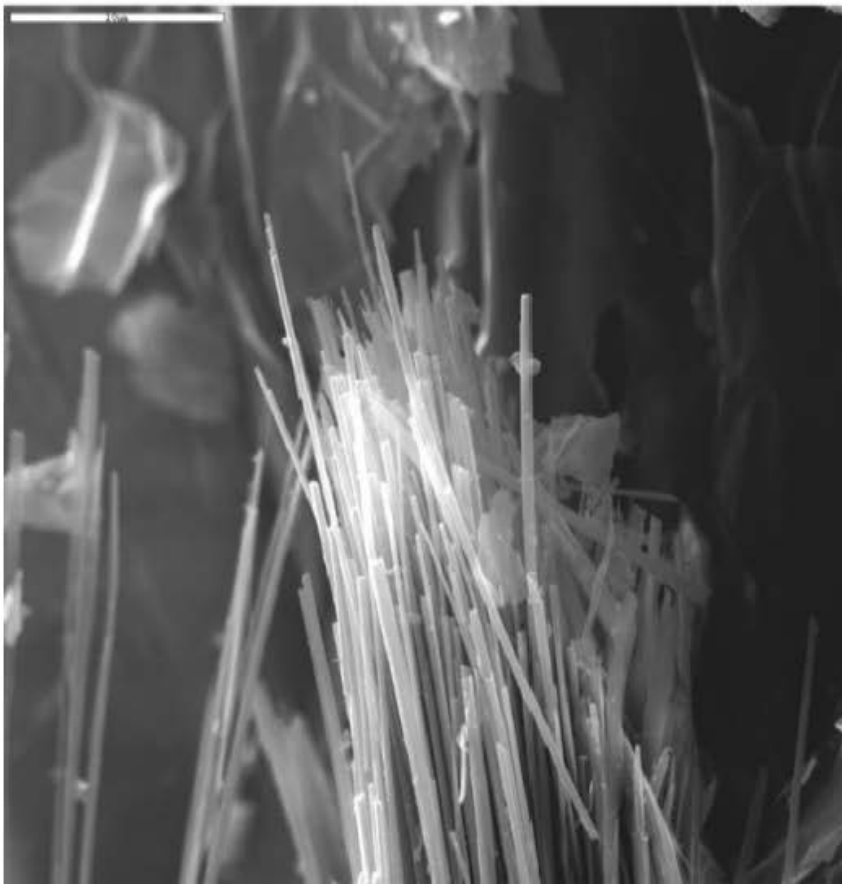
▲ FIGURE 3.34 Asbestiform amphibole fibers from Libby Montana. Source: Photo courtesy of Greg Meeker, U.S. Geological Survey.
