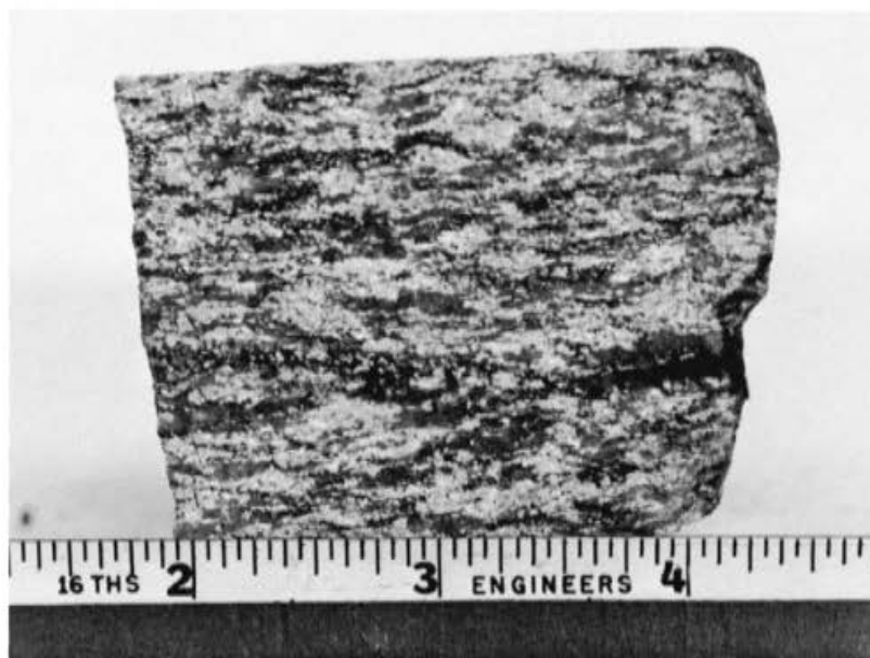
◀ FIGURE 6.11 Gneiss, a coarse-grained metamorphic rock, with broad light- and dark-colored bands of foliation (Ferry County, Washington). Source: R. L. Parker; photo courtesy of U.S. Geological Survey.
