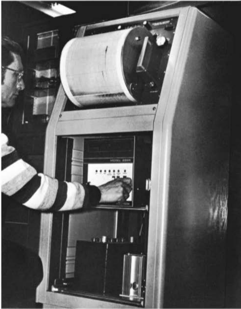
◀ FIGURE 8.37 A seismograph is the instrument used to measure seismic waves. Source: Photo courtesy of U.S. Geological Survey.
