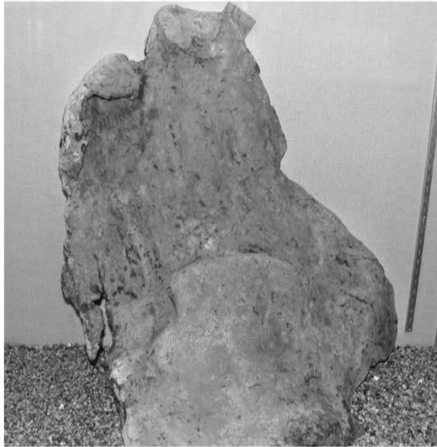
▲ FIGURE 3.30 Large clast of native copper from the Upper Peninsula of Michigan. In elemental form, copper is weak and malleable. This clast, which is approximately 0.75 m in height, was deformed during erosion and transport by a glacier. Source: Photo courtesy of the author.
