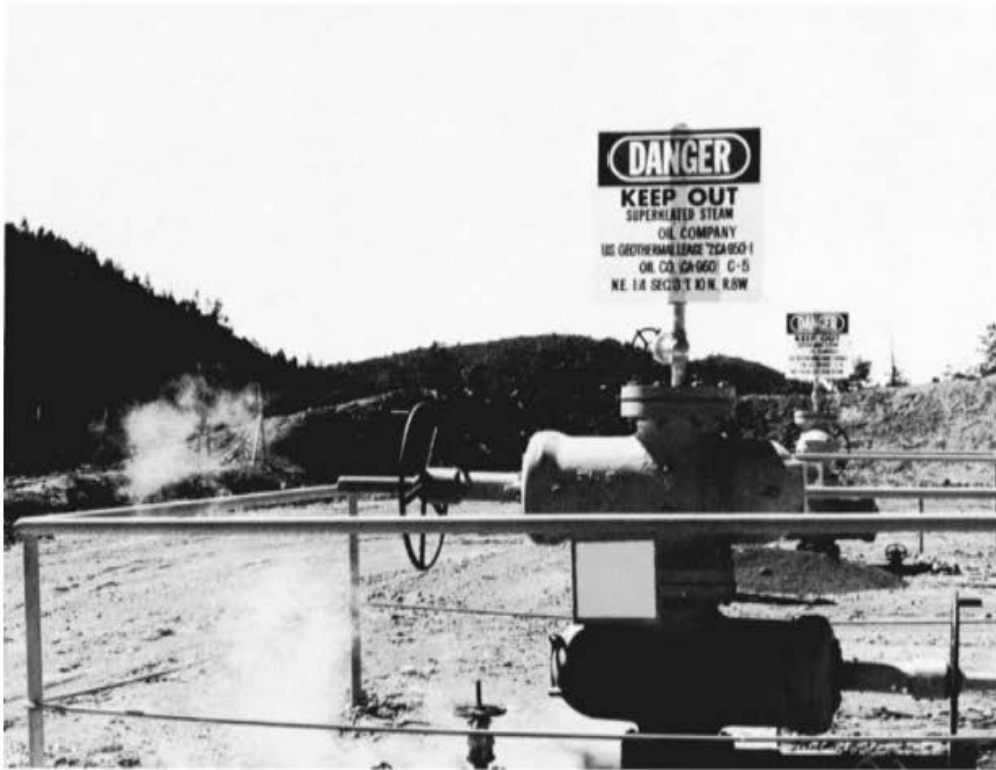
▲ FIGURE 2.11 Steam wells at The Geysers geothermal area, California. Source: Photo courtesy of U.S. Geological Survey.
