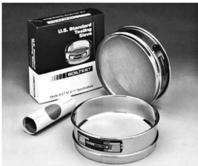
◀ FIGURE 10.10 Sieves used for determining grain-size distribution of soil. Source: Photo courtesy of Soiltest Inc.
