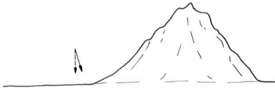
▲ FIGURE 2.18 Horizontal deflection of a plumb bob by the mass of a prominent mountain range.
