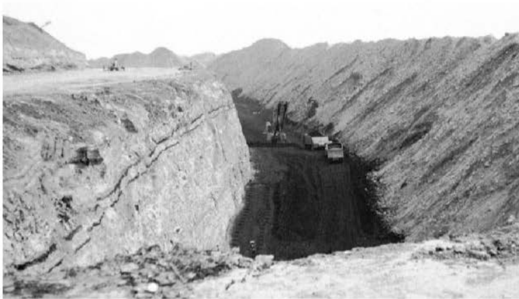
▲ FIGURE 1.21 Extraction of coal from an open-pit mine in central North Dakota. About 20 m of overburden has been removed above the coal bed.
