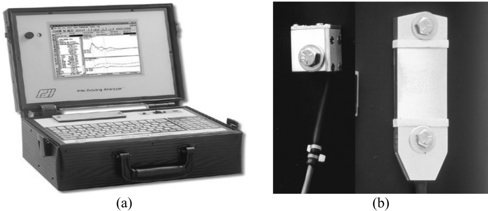
Figure 11.7. (a) Pile-driving analyzer; (b) Accelerometer (left) and strain gage (right) mounted near the top of a pile to provide input to the pile-driving analyzer (Pile Dynamics Inc., http://web.pile.com/pdi/default.asp?Company=PDI ).
