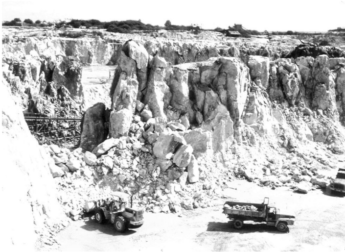
Figure 14.5. Highly irregular or pinnacled limestone bedrock, Sunway mine/quarry, Subang Jaya, Selangor Malaysia (now Bandar Sunway).
