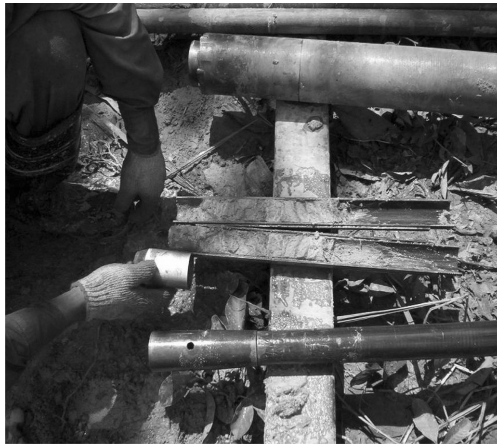
Figure 3.5. Split tube sampler for obtaining samples from SPT tests.
