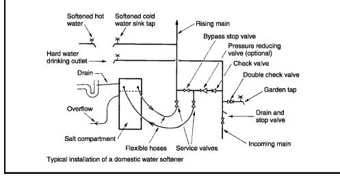
Domestic sanitary appliances – all potable (drinkable) water supplies must be protected against pollution by backflow or back siphonage from water that could be contaminated. Protection is effected by leaving sufficient space or air gap between the lowest point of the control device or tap discharge and the appliance spill over level.
