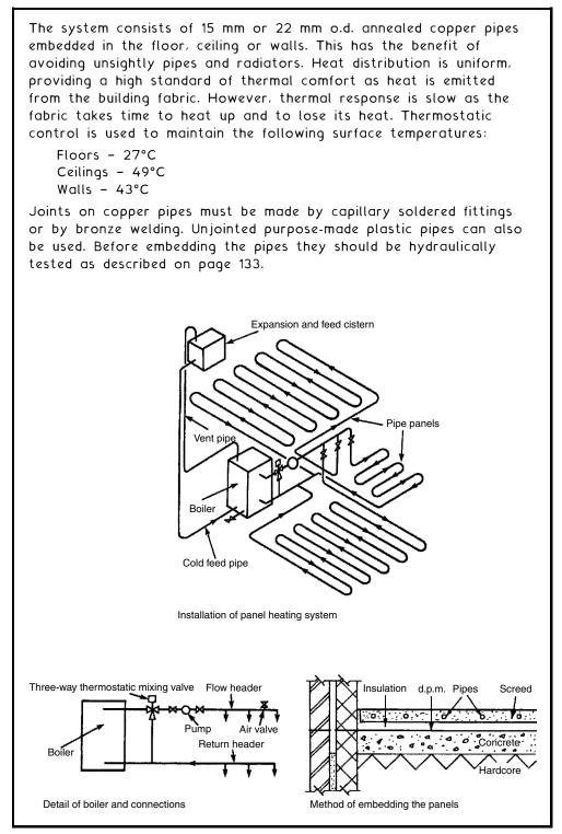
Current practice is to use jointless plastic pipe in continuous coils. Pipes can be embedded in a 70 mm cement and sand screed (50 mm minimum cover to tube). In suspended timber floors the pipe may be elevated by clipping tracks or brackets with metallic reflective support trays, prior to fixing the chipboard decking. Materials include:
