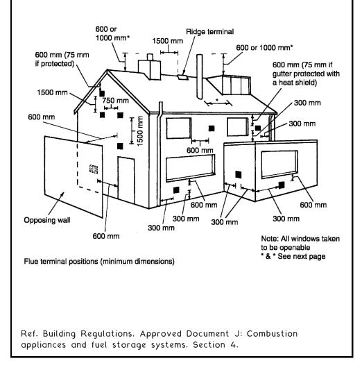
The following guidance provides minimum acceptable dimensions with regard to appliance efficiency, personnel and fire safety. The listing should be read with the illustration on the previous page. Local conditions such as wind patterns may also influence location of terminals. Flue terminal guards may be used as a protective barrier where direct contact could occur.
