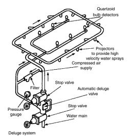
Multiple control system – a heat sensitive sealed valve controls the flow of water to a small group of open sprayers attached to a dry pipe. When a fire occurs, the valve quartzoid bulb shatters allowing the previously retained water to displace the valve stem and flow to the sprayers. An alternative to a heat sensitive valve is a motorised valve activated by a smoke or fire detector.
