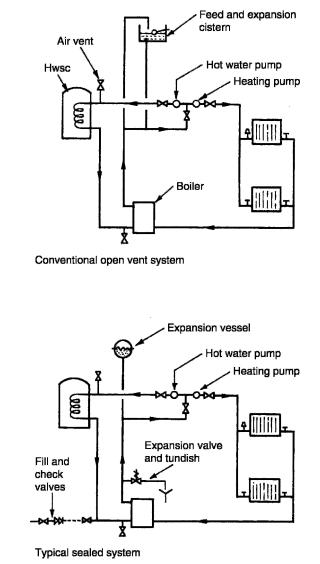
In conventional low pressure systems, air and other gases produced by heating water should escape through the vent and expansion pipe. Air must be removed to prevent the possibility of air locks, corrosion and noise. To assist air removal, a purpose-made device resembling a small canister may be used to concentrate the gases. This simple fitting is located on the boiler flow and vent pipe to contain the water velocity and ensure efficient concentration and release of air into the vent.
