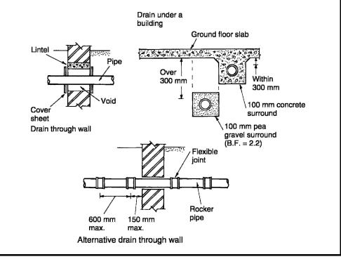
Rigid jointing of clay drain pipes is now rarely specified as flexible joints have significant advantages:
