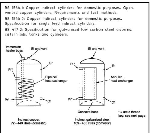
Direct cylinders have no coil or annular heat exchangers. They can be identified with female pipe threads for the primary flow and return connections. For domestic use: copper – 74 to 450 litres capacity, galvanised steel – 73 to 441 litres capacity. Direct and indirect cylinders for industrial and commercial applications are manufactured in copper and galvanised steel in capacities up to 4500 litres.
