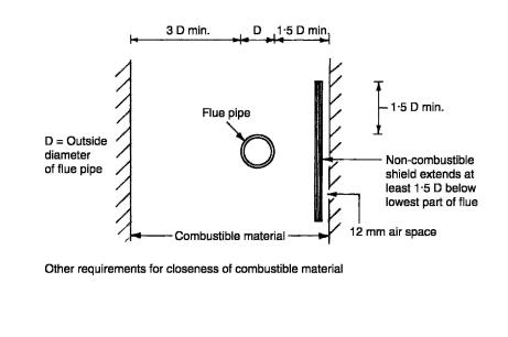
Flue outlets must be above the roof line to effect clear, unhindered dispersal of combustion products without creating a fire hazard. See `Open Fire Places and Flues' in the *Building Construction Handbook*.
