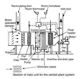
Notes: (1) Pre-heater coil may be used with chilled water as a cooler in the summer months, but two separate coils are usually fitted.
