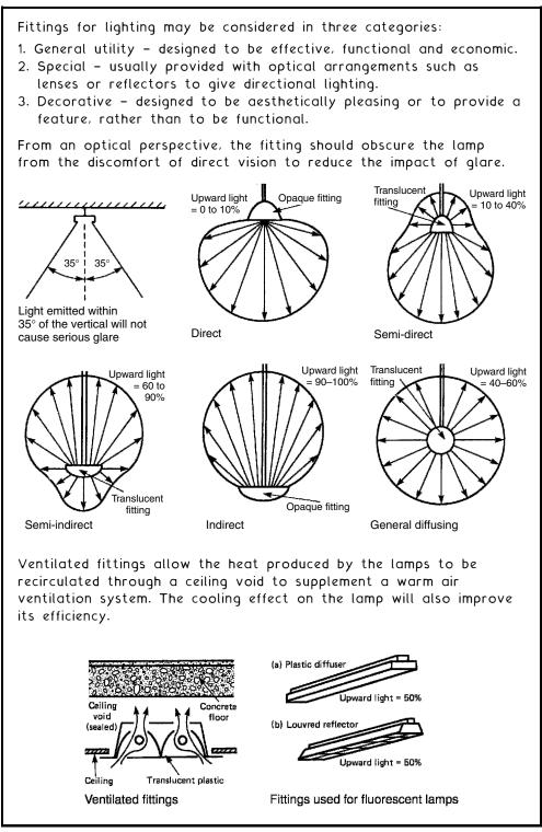
Luminaire – a word to describe the complete lighting unit including the lamp. When selecting a lamp type, it is important to select a luminaire to complement the lamp both functionally and aesthetically. A luminaire has several functions: it defines the lamp position, protects the lamp and may contain the lamp control mechanism. In the interests of safety it must be well insulated, in some circumstances resistant to moisture, have adequate appearance for purpose and be durable.
