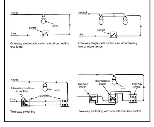
The purpose of a `master' switch is to limit or vary the scope of control afforded by other switches in the same circuit. If a `master' switch (possibly one with a detachable key option) is fixed near the main door of a house or flat, the householder is provided with a means of controlling all the lights from one position.
