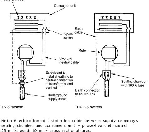
Pages 380, 381 and 385 show that the consumer's earth conductor is connected to the neutral and earthed at the local transformer. For below ground supplies this arrangement provides a path of low resistance for an electrical fault. With an overhead supply typical of rural areas, individual consumers must provide a suitable earth terminal or electrode as shown on page 384.
