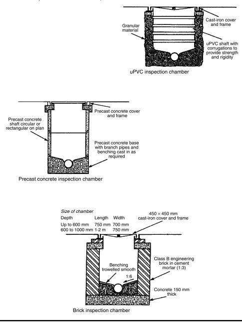
The term manhole is used generally to describe drain and sewer access. By comparison, manholes are large chambers with sufficient space for a person to gain access at drain level. Where the depth to invert exceeds 1 m, step irons should be provided at 300 mm vertical and horizontal spacing. A built-in ladder may be used for very deep chambers. Chambers in excess of 2.7 m may have a reduced area of access known as a shaft (min. 900 × 840 mm or 900 mm diameter), otherwise the following applies:
