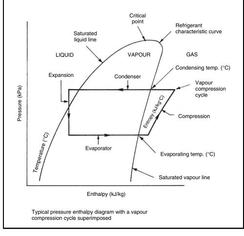
Efficient operation of refrigeration systems depends to a large extent on maintaining condenser temperature at an optimum level. This is necessary for correct reaction of the refrigerant. The cooling medium can be water or air. Water is more effective, but for practical purposes and health issues (see page 205), air cooling is becoming more widely used.
