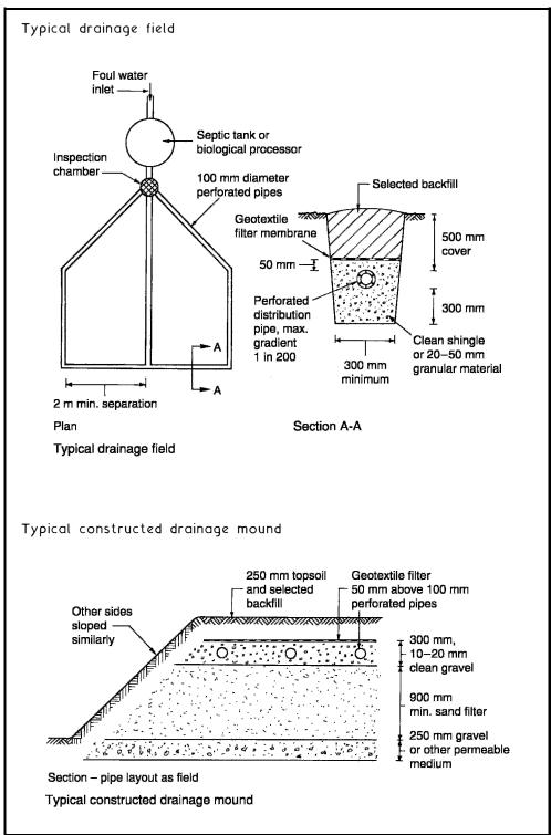
These provide a natural method for secondary treatment of sewage from septic tanks or biological processing equipment.
