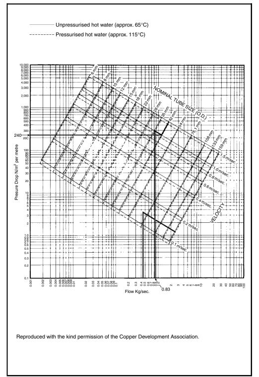
Circulatory pumps produce minimal pressure in the primary flow and return, but the flow rate is considerably enhanced. The pressure can be ascertained from design charts as a pressure drop in  $N/m^2$  per metre or pascals per metre.  $1 N/m^2$  equates to 1 pascal (Pa).
