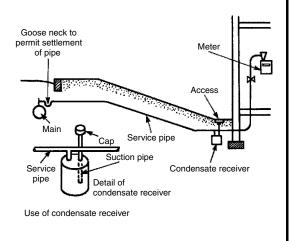
A service pipe is the term given to the pipe between the gas main and the primary meter control. A polyethylene pipe is used underground and steel or copper pipe where it is exposed. Wherever possible, the service pipe should enter the building on the side facing the gas main. This is to simplify excavations and to avoid the pipe having to pass through parts of the substructure which could be subject to settlement. The service pipe must not:
