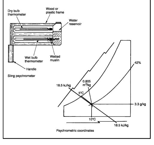
Treatment of air is based on heating, cooling, humidification and dehumidification. These processes can be represented by lines drawn on the psychrometric chart.
