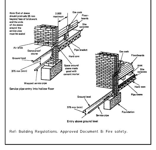
Gas service pipe risers must be installed in fire protected shafts constructed in accordance with the Building Regulations, Approved Document B: Fire safety. Possible methods for constructing a shaft include:
