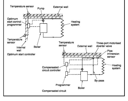
Weather compensated circuit – accurate control of indoor temperature depends on monitoring and modulating system heat input with the heat losses from a building. This differs considerably from the traditional heating system controlled solely by a thermostat. A thermostat functions relative to internal air temperature, switching on the boiler to supply water at a pre-set temperature.
