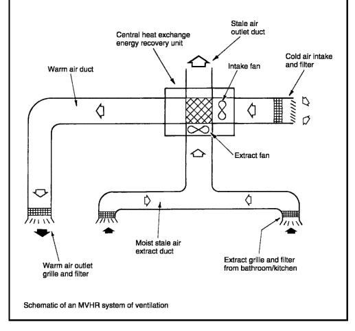
Mechanical ventilation systems are frequently applied to commercial buildings, workshops, factories, etc., where the air change requirements are defined for health and welfare provision. There are three categories of system:
