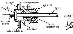
Section of termination joint for mineral insulated copper covered cable (MICC)
