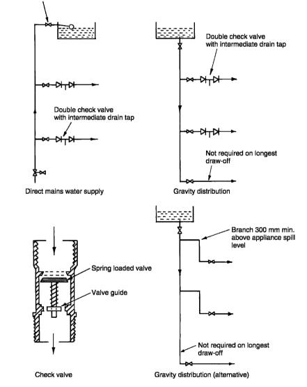
Mains water supply to commercial and industrial premises must be protected against the possibility of contamination by backflow. Where toxic processes exist, e.g. dyeing, chemical manufacture, insecticide preparation, car washing, irrigation systems, etc., it is imperative that the effects of a pressure reduction on drinking water supplies be contained.
