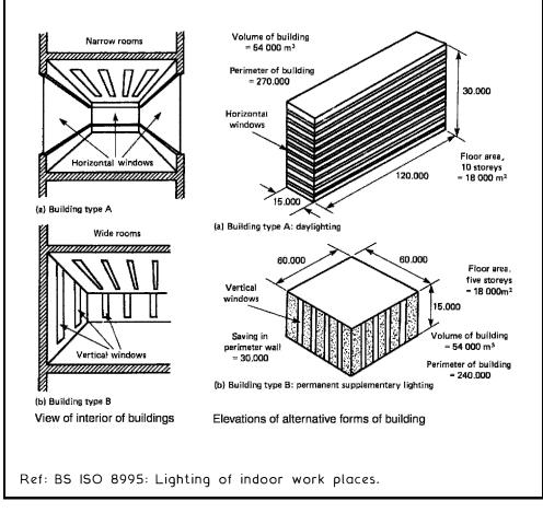
The daylight received inside a building can be expressed as `the ratio of the illumination at the working point indoors, to the total light available simultaneously outdoors'. This can also be expressed as a percentage and it is known as the `daylight factor'.
