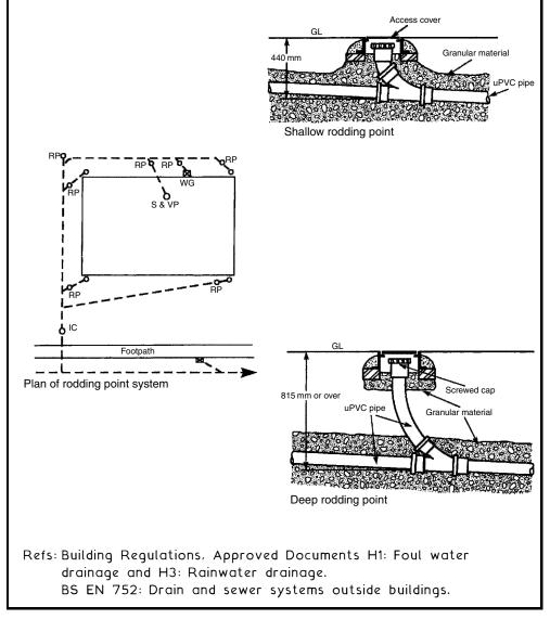
Connections between drains and sewers must be obliquely in the direction of flow. Drains may be connected independently to the public sewer so that each building owner is responsible for the maintenance of the drainage system for that building. In situations where there would be long drain runs, it may be more economical to connect each drain to a private sewer. This requires only one sewer connection for several buildings. Maintenance of the private sewer is shared between the separate users.
