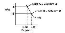
• Velocity reduction – air velocity is selected for the main section of ductwork and reduced for each branch. For example, selected air velocities for ducts A and B are 8 m/s and 5 m/s respectively:
