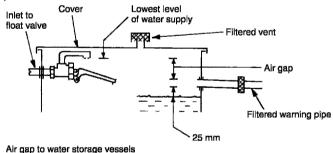
In this situation the air gap should be ≥20 mm or 2×internal diameter of the regulating valve inlet orifice (take greater value). For example, a 20 mm internal diameter orifice: 20 mm or 2×20 mm = 40 mm. Air gap = 40 mm minimum. Refs: Water Supply (Water Fittings) Regulations. BS EN 1717: Protection against pollution of potable water in water installations and general requirements of devices to prevent pollution by backflow.
