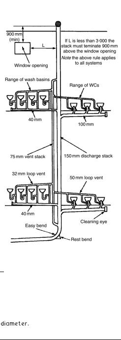
This system was devised to comply with the old London County Council requirements for connection of soil (WC and urinal) and waste (basin, bath, bidet, sink) appliances to separate stacks. For modern systems the terms soil and waste pipes are generally replaced by the preferred terminology, discharge pipes and discharge stacks.
