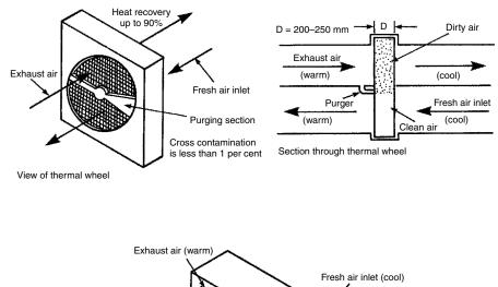
Exhaust air (warm) Fresh air inlet (cool) Fresh air inlet (warm) Exhaust air (cool)
