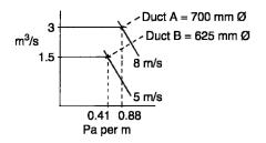
• Equal friction/constant pressure drop – air velocity is selected for the main section of ductwork. From this, the friction is determined and the same figure applied to all other sections. For example, selected air velocity through duct A is 7 m/s:
