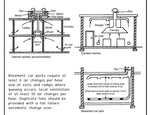
Fan assisted ventilation systems supplying external air to habitable rooms must have a facility to pre-heat the air. They must also have control over the amount of air extracted, otherwise there will be excessive heat loss. A mechanical inlet and mechanical extract system can be used to regulate and balance supply and emission of air by designing the duct size and fan rating specifically for the situation.
