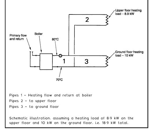
The size of pipework can be calculated for each sub-circuit and for the branches to each emitter. Unless emitters are very large, 15 mm o.d. copper tube or the equivalent is standard for connections to radiators in small bore installations. To illustrate the procedure, the drawing on the previous page allows for calculation of heating flow and return pipes at the boiler, and the supply pipes to each area of a house.
