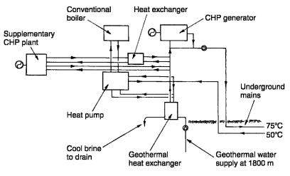
Schematic combined geothermal, CHP and conventional boiler district heating system
