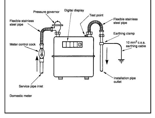
Gas meters measure the volume of gas in cubic feet or cubic metres consumed within a building. The discharge is converted to kilowatt-hours (kWh). 100 cubic feet or 2.83 cubic metres is approximately 31 kWh, (see page 374). Some older meters have dials but these have been largely superseded by digital displays which are easier to read.
