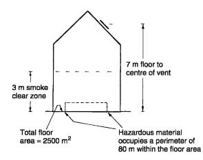
By interpolation, ventilation factor for 7 m approximates to 0.41 m. Ventilator area can be taken as the perimeter occupied by hazardous material, multiplied by the ventilation factor, i.e. 80 m  $\times$  0.41 m. This approximates to 33 m<sup>2</sup> or (33/2500  $\times$  100/1) = 1.3% of the floor area.
