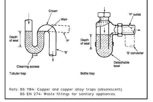
The most obvious cause of water seal loss is leakage due to defective fittings or poor workmanship. Otherwise, it may be caused by poor system design and/or installation:
