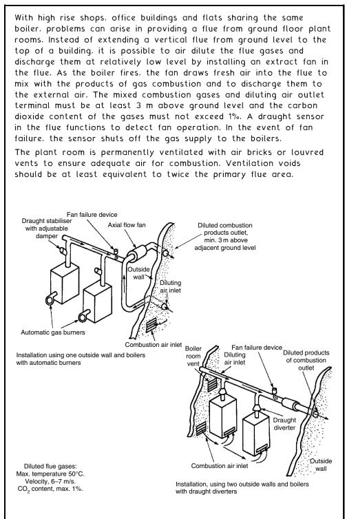
Fan assistance with the dilution and removal of combustion products has progressed from commercial and industrial applications in open flues, to domestic appliance balanced flues. In addition to diluting the  $CO_2$  content at the flue gases point of discharge, fanned draught balanced flue systems have the following advantages over standard balanced flues:
