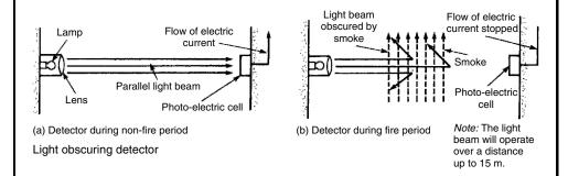
Laser beam – a band of light which can be visible or infra-red projected onto a photo-electric cell. It does not fan out or diffuse as it travels through an uninterrupted atmosphere. The beam can operate effectively at distances up to 100 m. If a fire occurs, smoke and heat rises and the pulsating beam is deflected away from the cell or reduced in intensity. As the cell is de-energised, this effects on alarm relay.
