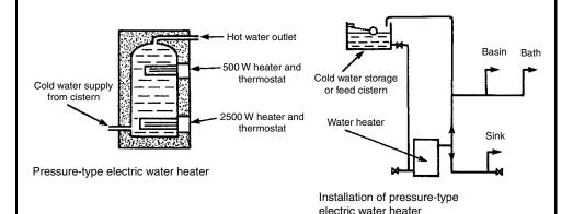
Immersion heaters – safety cut-out. Since 2004, immersion heater manufacturers are required to incorporate an additional integral safety device, independent of the main thermostat. This brings immersion heaters for vented water heating into line with the requirements for unvented water heaters.
