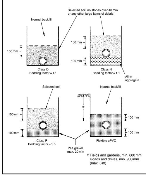
Drain trenches should be avoided near to and lower than building foundations. If it is unavoidable and the trench is within 1 m of the building, the trench is filled with concrete to the lowest level of the building. If the trench distance exceeds 1 m, concrete is filled to a point below the lowest level of the building equal to the trench distance less 150 mm.
