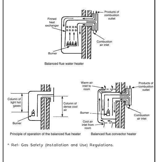
Balanced flue terminals must be positioned to ensure a free intake of air and safe dispersal of combustion products. Generally, they should be located on a clear expanse of wall, not less than 600 mm from internal or external corners and not less than 300 mm below openable windows, air vents, grilles, gutters or eaves.
