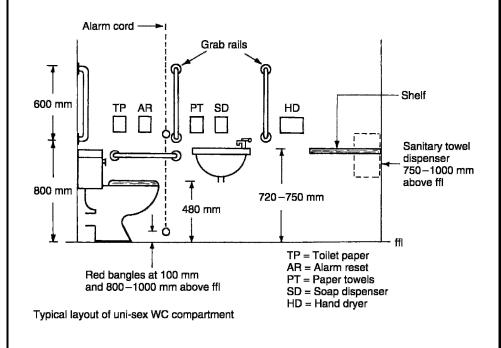
Facilities for ambulant (not confined to a wheelchair) disabled people should be provided within conventional separate sex WC and washroom compartments. A suitable compartment will contain some appliances specifically fitted with support rails. There should also be sufficient space to accommodate persons with impaired leg movement and with crutches. Other provisions and facilities in buildings other than dwellings:
