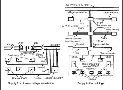
Note: For easy identification, each phase cable has colour coded plastic insulation of brown (red), black (yellow) or grey (blue). The neutral is colour coded blue (black). An outer sheathing of red or black provides for future identification. Older installations will have colour codes as indicated in brackets.
