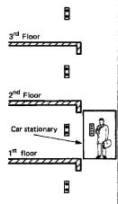
Passenger enters the car and press buttons to travel upwards
