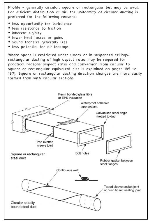
Galvanised sheet steel is the most common material used for ventilation and air conditioning ducting. Factory prefabricated sections are site jointed by bolted steel angle flanges with a rubber sealing gasket, the rigid angles can also function as suspended bracket fixings. Sleeve jointing with pop-rivets and tape sealant is also used with smaller profile sections.
