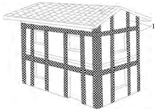
FIGURE 32.26 Strengthening by splint and bandage technique (IS 13935: 1993).
