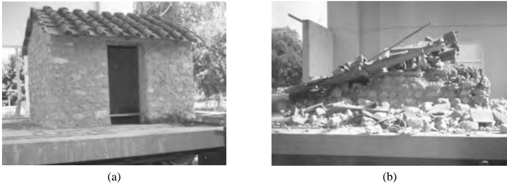
FIGURE 31.4 (a) Model 1 (unstrengthened) under shock test (b) Complete collapse of model 1 at shock E-23.
