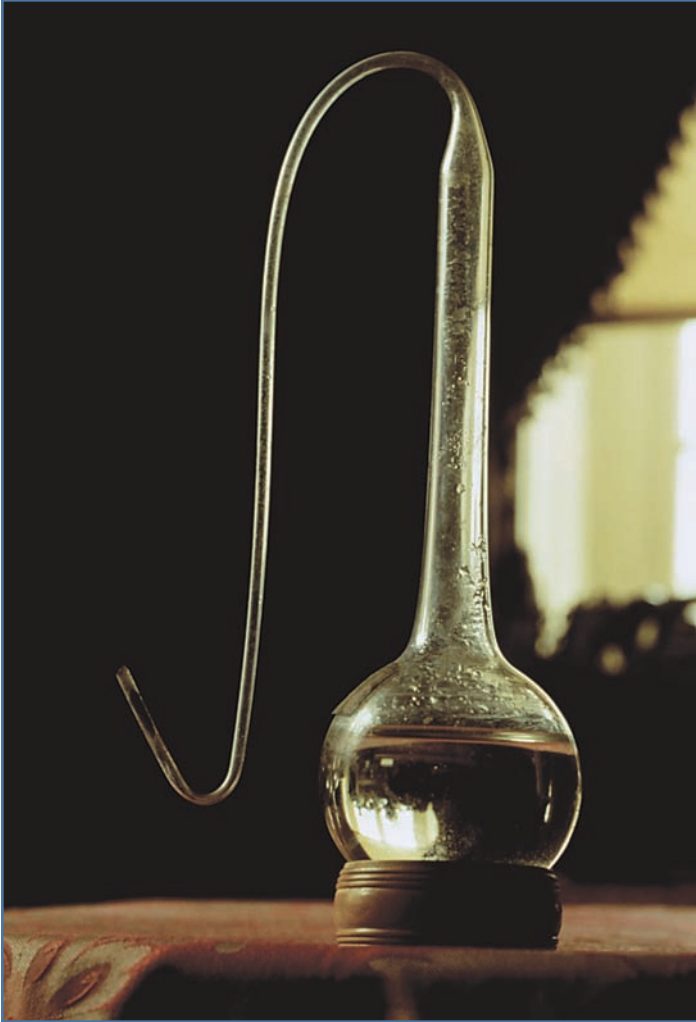
Figure 2.1 A swan-neck flask such as this one was used by Louis Pasteur to disprove the theory of spontaneous generation. The experiment led to the establishment of Koch's postulates.
