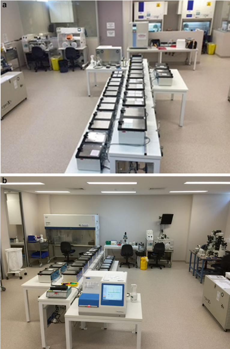
Fig. 7.4 (a, b) Incubators face towards an internal culture access system (incubators, workstations, ICSI areas). Staff access for areas not involved with embryo culture (i.e. embryo transfer rooms, culture media preparation areas, media equilibration incubators, fridges, and sperm preparation areas), happens on the other side of the incubator bench (photo courtesy of IVFAustralia)
