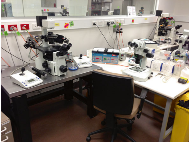
Fig. 7.2 Work-pod in a standard air laboratory. Bench-top incubator to use at work-pod, ICSI microscope and Dissecting microscope workbench, all located together for minimal dish and staff movement (photo courtesy of Melbourne IVF)
