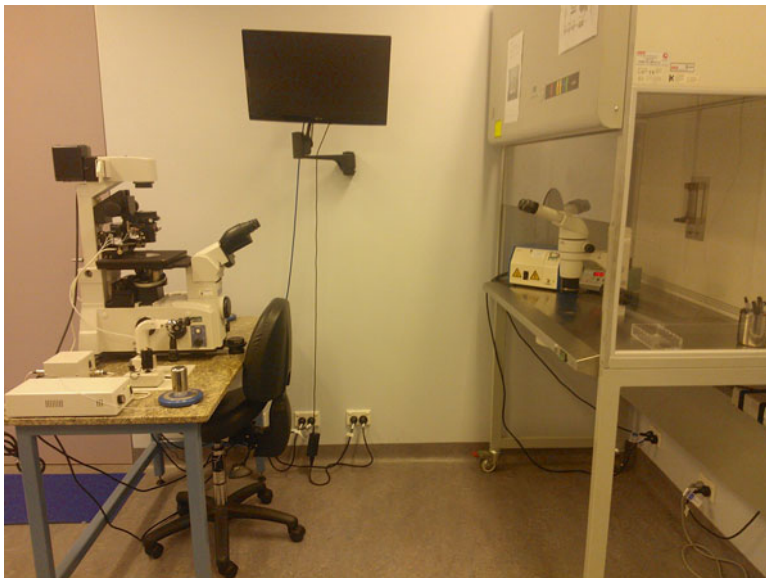
Fig. 7.3 Single person work area in a standard air laboratory, incorporating an ICSI microscope, a Dissecting microscope, and K-Systems workbench all located close together, to eliminate staff movement behind you (photo courtesy of IVFAustralia)
