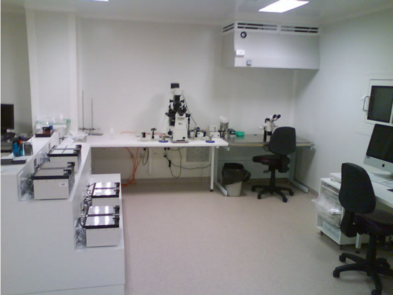
Fig. 7.1 Work-pod in an ISO14644 compliant clean room. Culture Incubators, ICSI microscope, Biopsy laser, Dissecting microscope, and K-Systems workbench are all located together for minimal dish and staff movement. Five work pods like this exist in a laboratory performing over 1800 fresh cycles (photo courtesy of IVFAustralia)
