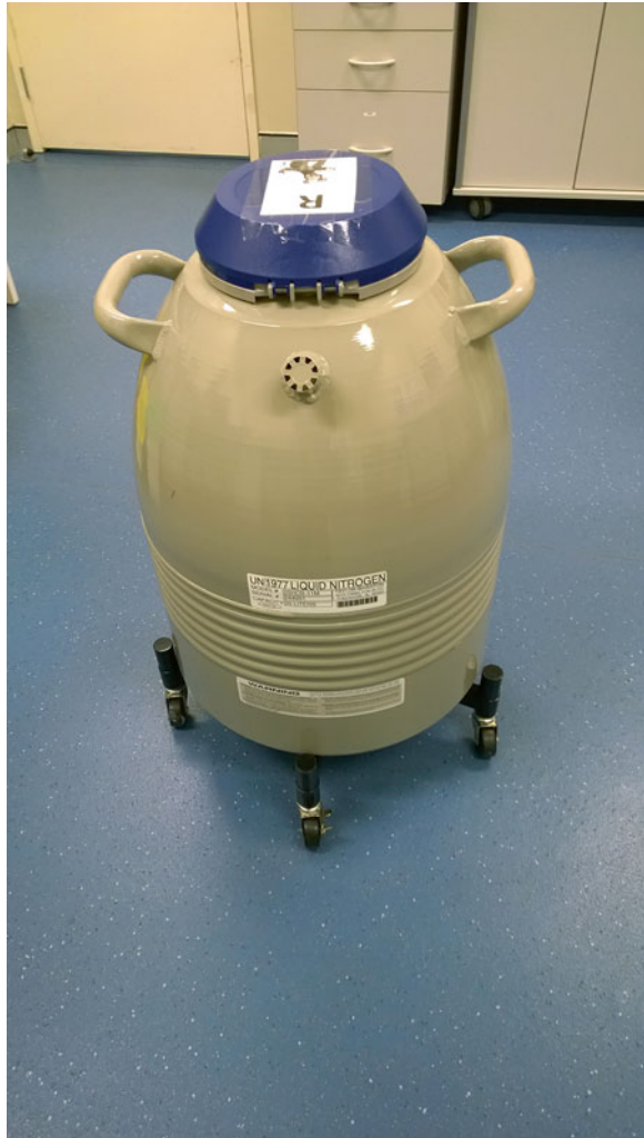
Fig. 8.3 Liquid nitrogen storage tank on roller base
