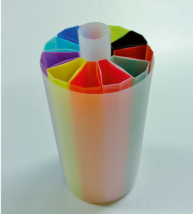
Fig. 8.5 An example of visotubes arranged in a maxi-goblet for storage of cryopreservation straws
