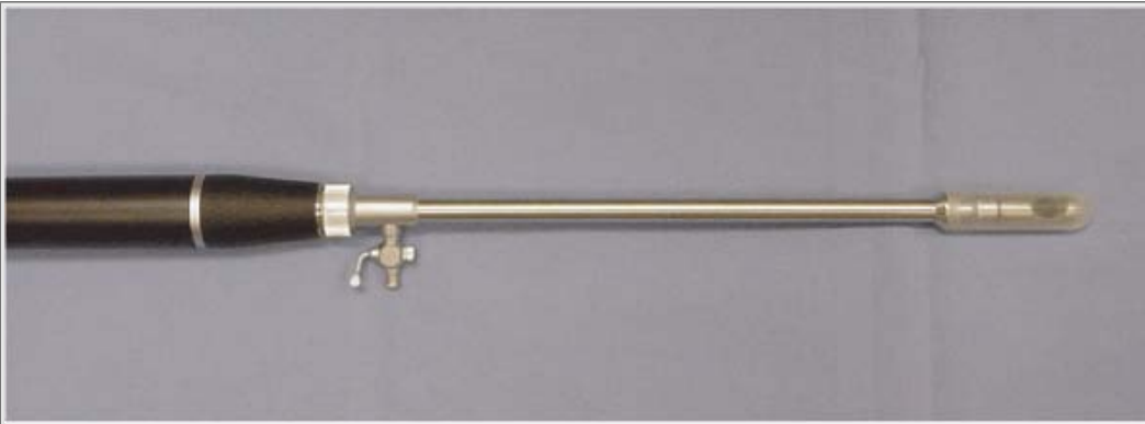
Figure 25.1 Bruel-Kjaer (Copenhagen, Denmark) ultrasound probe (type 1850) with a 7.0 MHz transducer (focal length, 2 to 5 cm) housed with a plastic cone.
