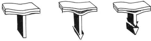
Figs 10.5B: Top edge of crura showing vulnerability to delamination like an inflatable 'I' beam.
