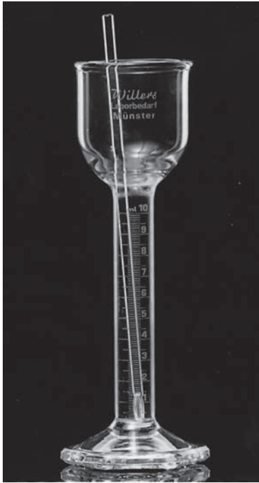
Fig. 9.1 Wide-mouthed, specially-made glass measuring cylinder and glass rod for the collection and mixing of semen and measurement of its volume
