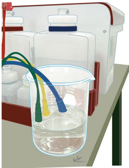
Fig. 24.32 Fluidic lines placed in 500 mL beaker of hot water before running decontamination cycle to clean the lines
