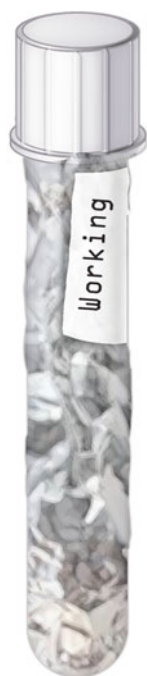
Fig. 21.1 Working luminol solution; wrapped in foil due to light sensitivity. [Reprinted with permission, Cleveland Clinic Center for Medical Art & Photography © 2015. All Rights Reserved]
