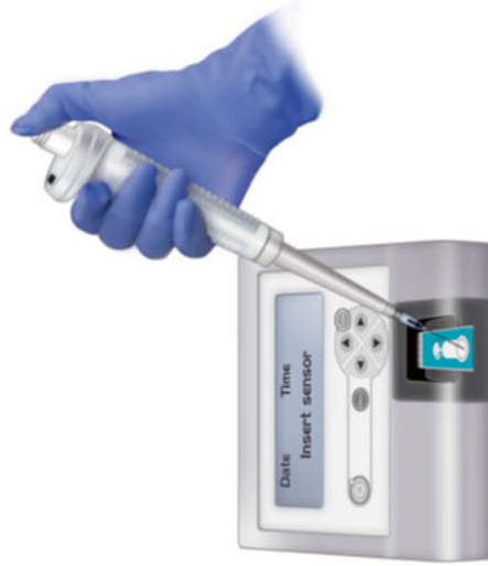
Figure 7. View of the sensor showing the application port for loading of the sample
