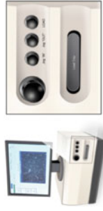
Figure 4. Front of CASA instrumentation; slide loading tray, jog in/out buttons, load button and focus knob.
