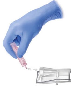
Figure 3. Two drops of sterile saline added to Cytofunnel of "blank" control slide.
