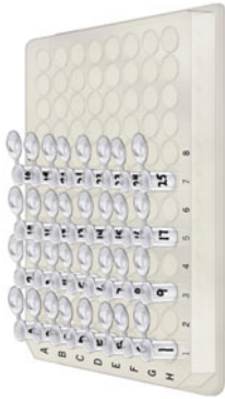
Figure 6. Samples A-G: reconstituted Trolox standards. Samples 1-25: diluted patient samples (10 \mu L patient seminal plasma + 90 \mu L assay buffer).
