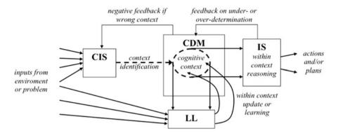
Fig. 9.1 How the context-identification system (CIS), the context-dependent memory (CDM), the local learning algorithm (LL), and Inference system (IS) might work together
