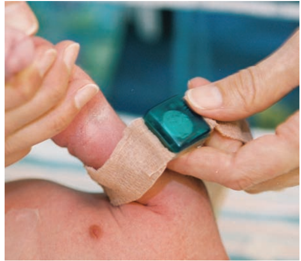
FIGURE 14.17 An example of a security sensor applied to a newborn's arm.
